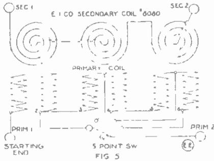
rent from leaking. Care should be exact used in connecting the secondary units, so that the current travels around the core always in the same direction.
