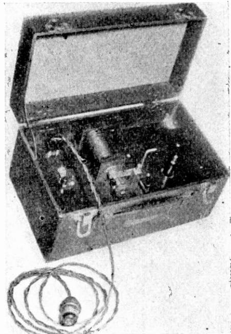
The 110 Volt Transformer and Secondary for the Oudin Coil
