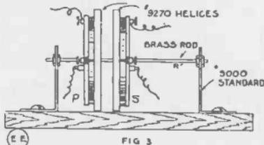
circuit with a smooth wave form. A small space usually exists between the two helices, when properly tuned. The connections for the oscillation transformer are shown at Fig. 4, for a spark coil transmitter. Here, A, is the aerial, G, the ground, HM, the hot-wire ammeter, anchor gap,
