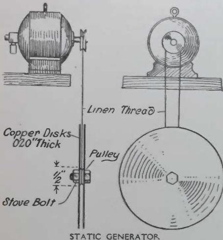
the pulley with the stove bolt as shown. Now make a belt of heavy linen thread. Place the thread over the pulley on the motor and set the disks' pulley upon the loop, thus leaving the disks suspended in the air. Start the motor, give the disks a turn and as soon as they come up to speed, they will act as a gyroscope and keep balanced.
