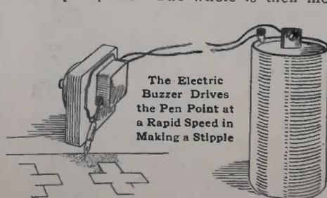
with the push button conveniently mounted on the opposite side. I found it better to mount the bell box upside down, making the stroke of the magnet or armature, when released, the working stroke of the pen. This
