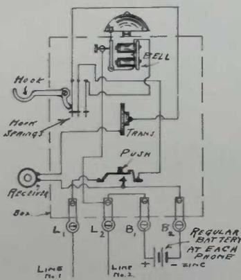
utilizing the ground as a conductor, in place of one wire; gas pipe or water pipe ground can be employed for this purpose. The push button on the instrument is not used in the combined system, but only the separate push buttons shown in diagram, which may be of the type sold by the E. I. Co. No. 1008, at six cents each.
