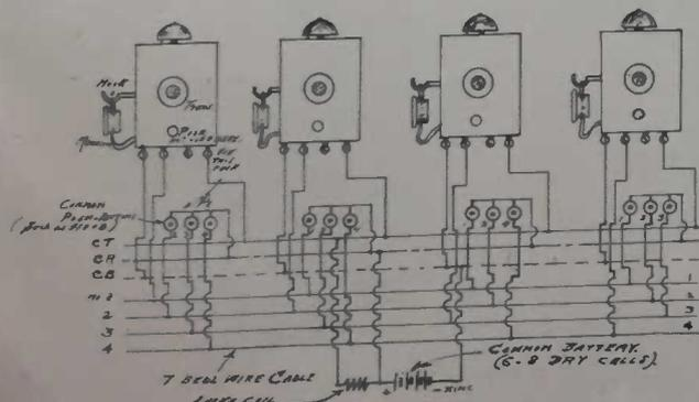
wet cells. The conductors used in the cable for this system may very well be No. 18 or 16 B. & S. cotton covered bell wire; and one of the wires of the system can be eliminated by
