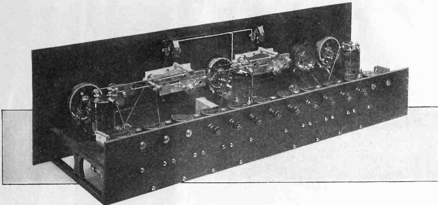
*Left hand rear end. Note the lug connection at the base of the transformer, and the condenser mounting*
