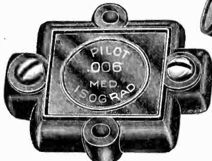
Because Pilot Isograd fixed Condensers are molded under tremendous pressure, they are completely sealed against heat, moisture and dust and hence are accurate, permanent and noiseless. Obtainable in capacities from .00025 to .015. Price from 35c to \$1.20.
