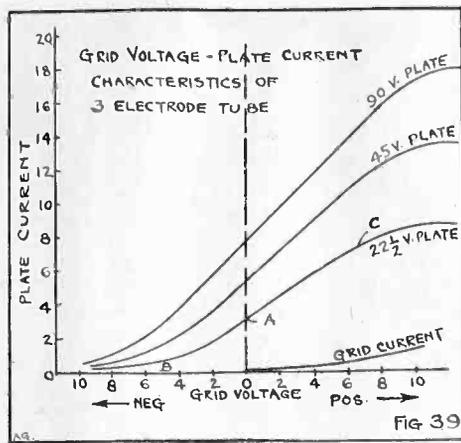
Fig. 39. With constant filament temperature, the filament-plate current depends upon the voltages on the grid and plate
