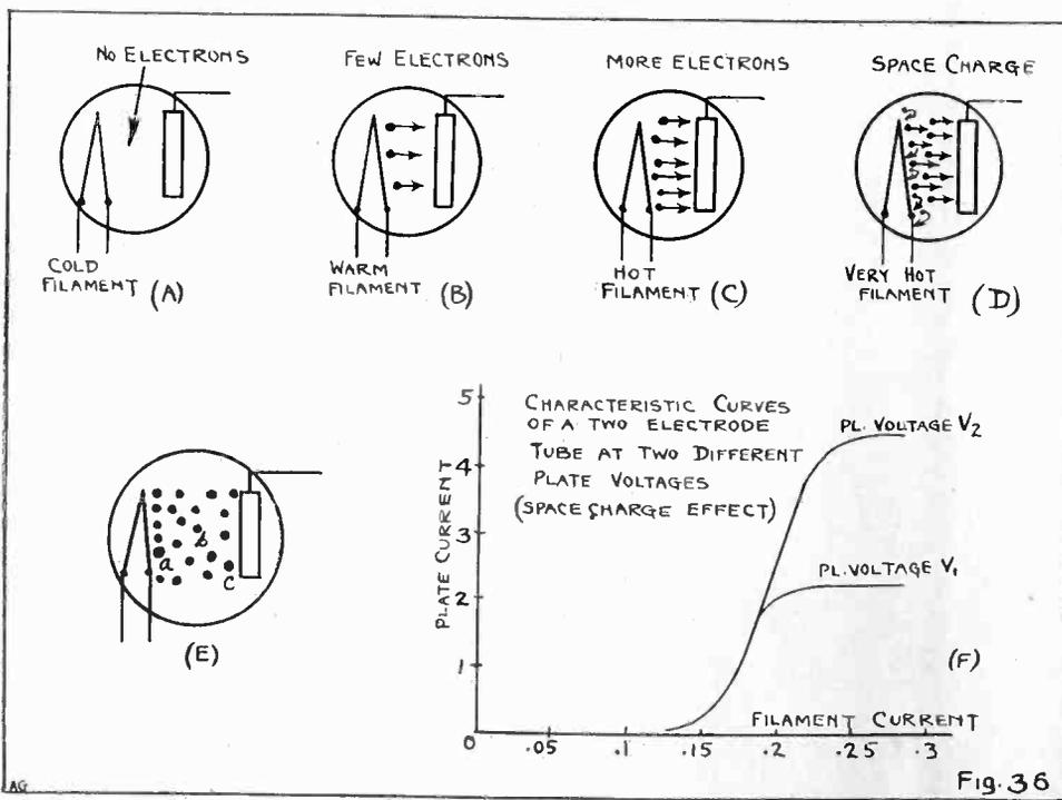
Fig. 36. The temperature of the filament controls the current flowing to the plate
