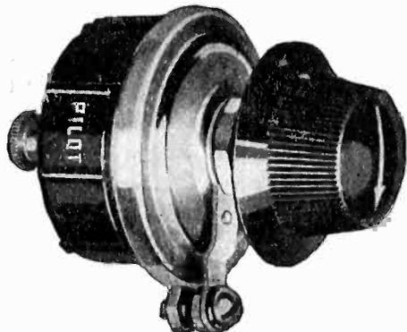
A non-inductive variable Resistor useful as Variable Grid Leak, Oscillation control in T.R.F. circuits, Volume and Regenerative control and as Regulator of voltage output in B Battery eliminators. Active compound is hermetically sealed in molded case. Range from practically zero to 30 megohms. \$1.25.
