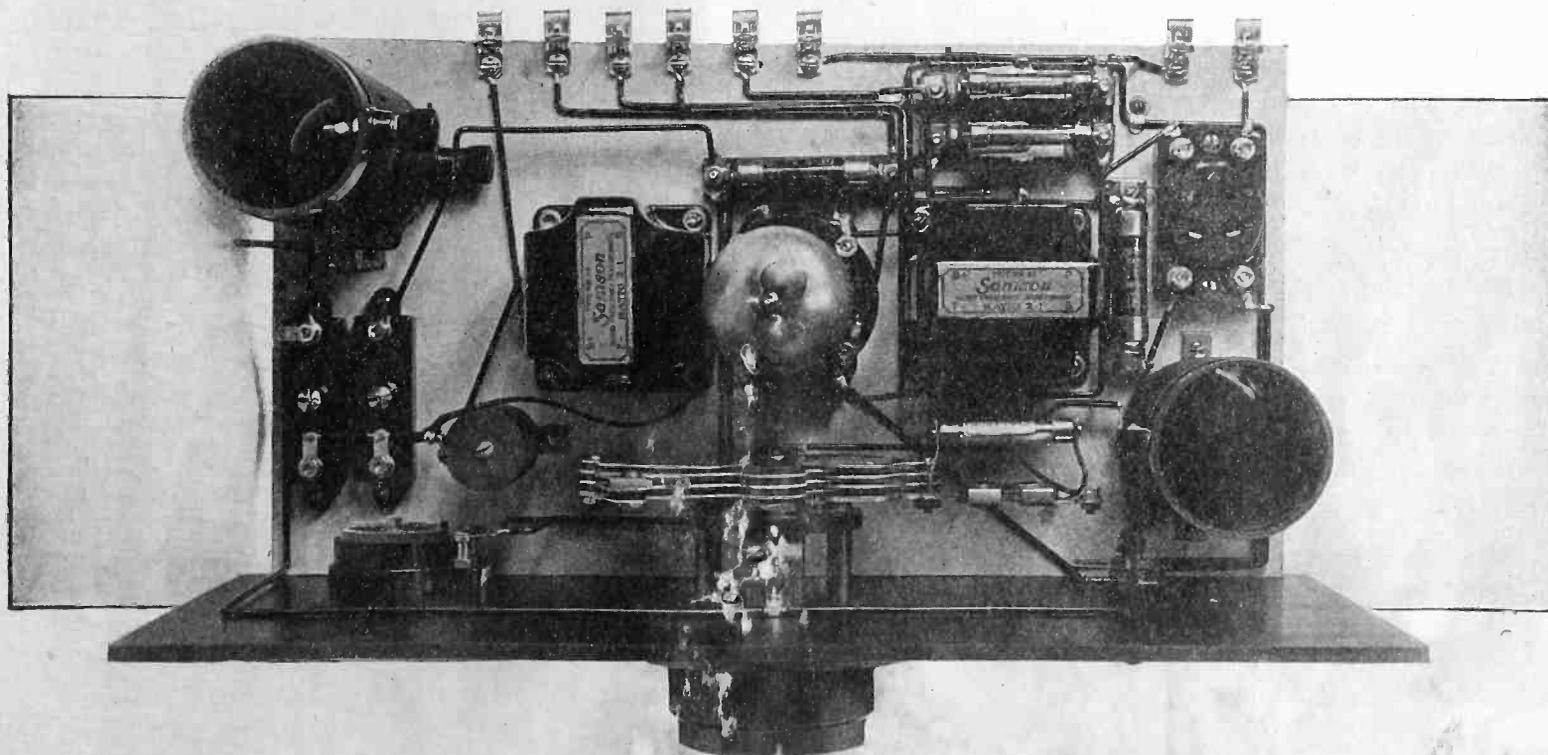
"Is this four-tube circuit obtained from two tubes by reflexing?" No, it is not. The heart of the N circuit, as described here, is the new Emerson Multivalve, which is really three tubes in one. This tube has three grids and three plates, and the filaments are wired in series so that the current consumption is the same as that of a standard 201-A type. You can readily appreciate that the addition of a power tube then gives four-tube efficiency and results with two-tube compactness and economy.
