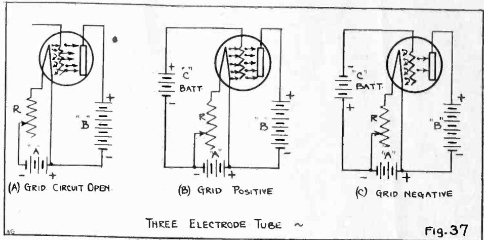
Fig. 37. What happens when a charge is put on the grid of a tube
