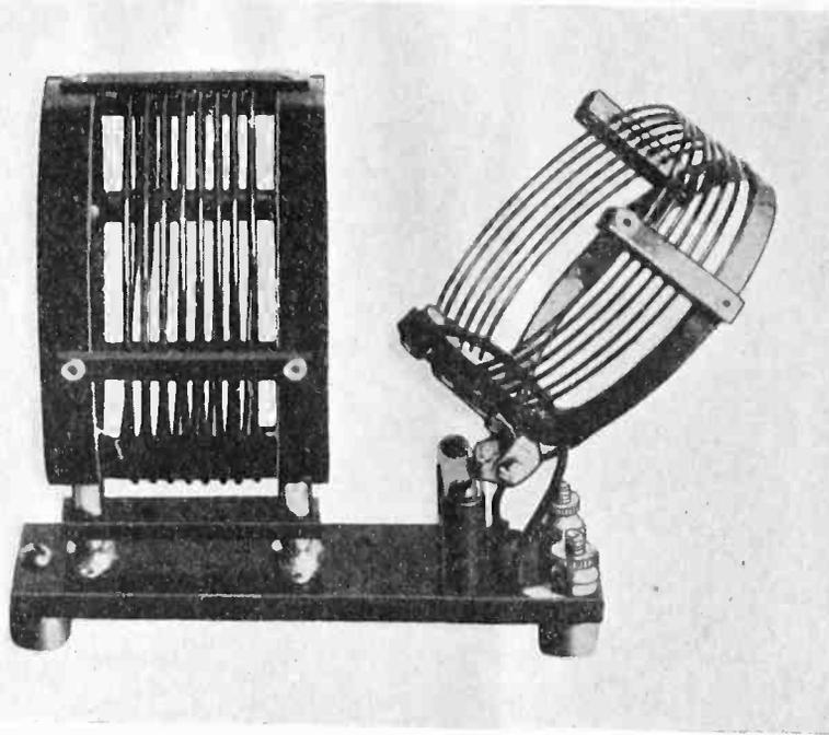
The antenna coupling unit. Several improvements have been made by the Aero company in the design of these coils
