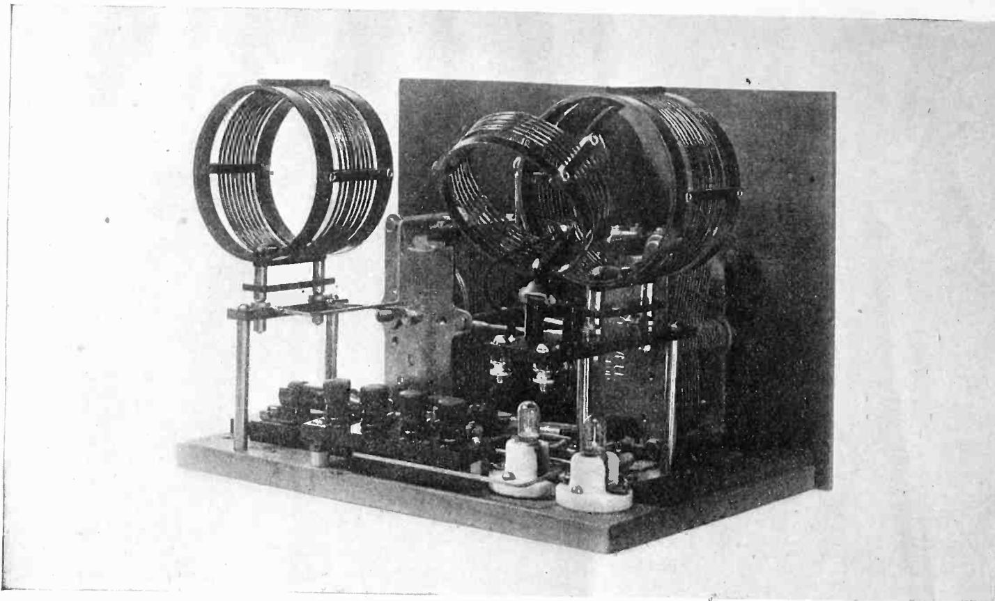
*Close-ups of the LP-SW transmitter. Combined with Bert Smith's S. W. receiver, it's the real thing for experimental communication*
