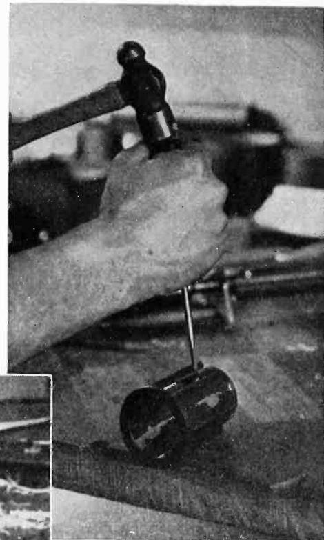
*At the right: Chipping out the thin wall, to start the hack-saw blade, after the holes have been drilled. Left: Cutting out the thin wall, close to the triangular strips. Center: A coil frame partly finished. A fairly fine file is best for this work, but it must be sharp, in order to cut the Bakelite. Be careful at all times not to split the end rings for much strain is put upon them while this work is in progress*
