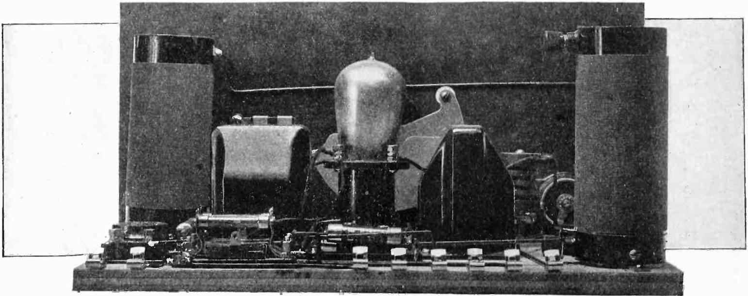
*Rear of the N circuit receiver. This shows the extra grid and plate terminals of the Multivalve*
