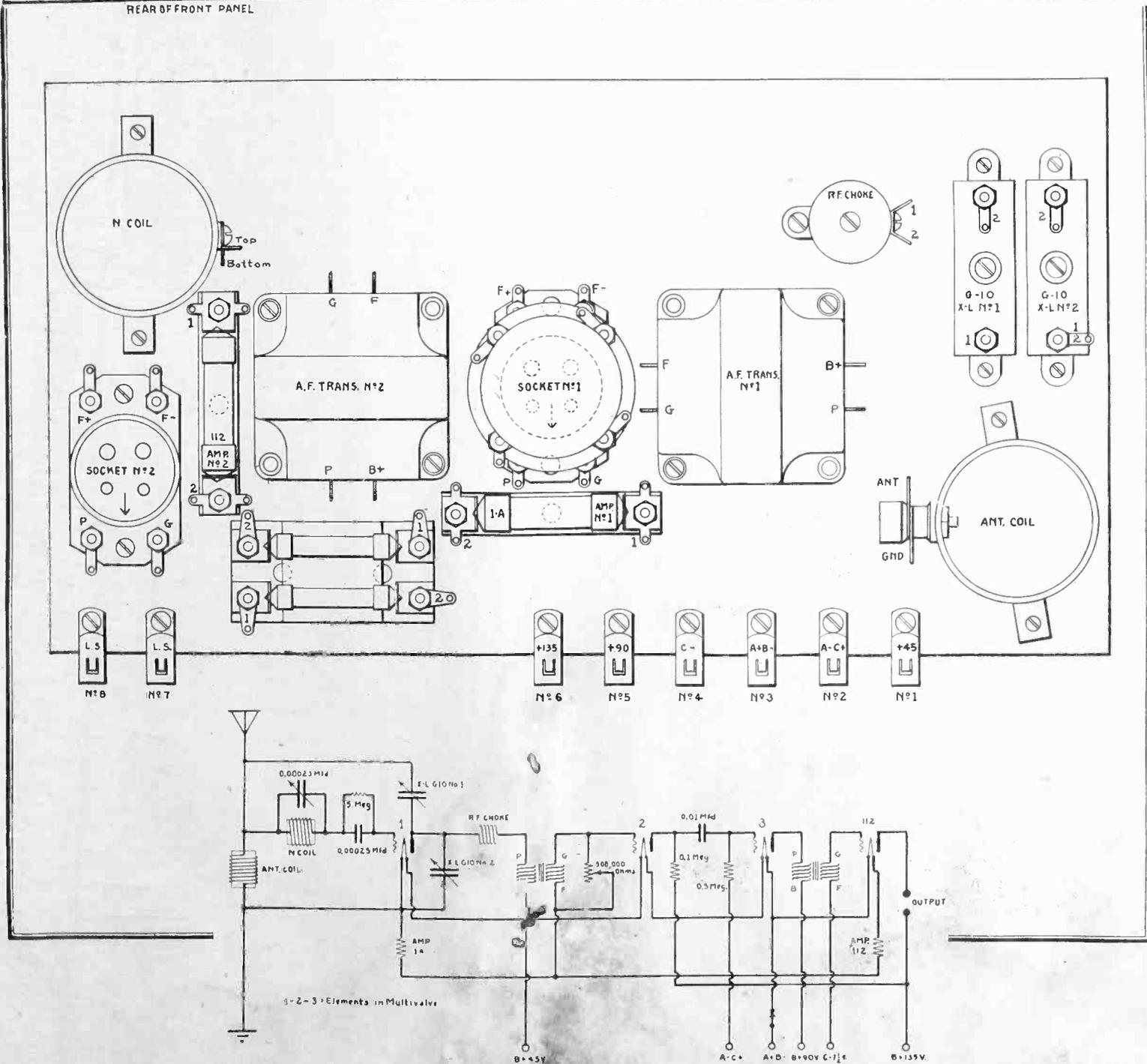
condenser No. 2 so that its capacity is at maximum. This is done by turning it to the right as far as it will go. Do not force it. Condenser No. 1 should be adjusted to minimum capacity by turning the screw to the left.
