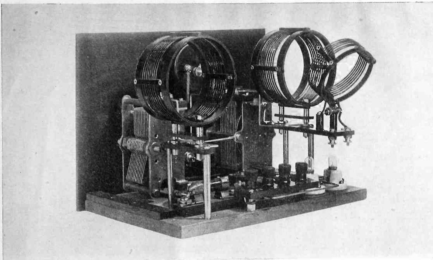
*Details of the coil mountings and the plug-in coils. Special spring friction plugs assure perfect contact to the jacks*
