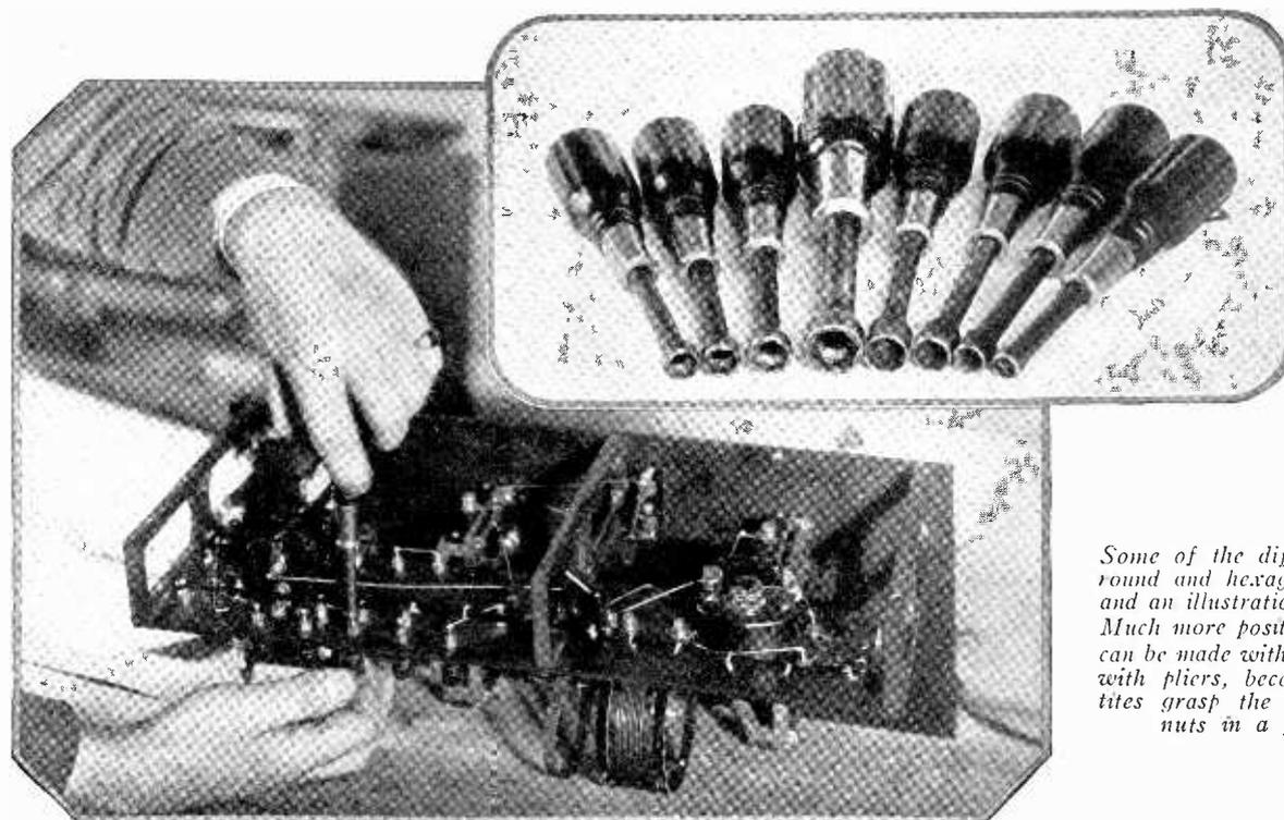
*Some of the different sizes of round and hexagonal Spintites, and an illustration of their use. Much more positive connections can be made with Spintites than with pliers, because the Spintites grasp the round or hex nuts in a firm grip*
