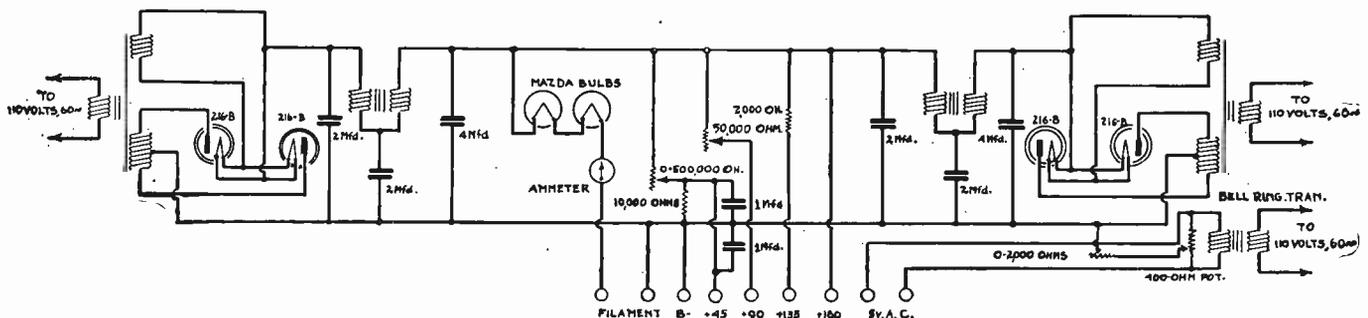
two unichokes, the filter and by-pass condensers, the bell ringing transformer, four UX sockets, two porcelain Mazda bulb sockets, four binding posts, a double resistor mount and a binding post strip. Before mounting any of the parts, draw a pencil line on the board parallel to the 12-in. edges, dividing it into two equal parts.
