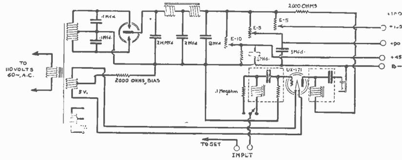
*Schematic diagram of the eliminator and power amplifier as G. H. Browning made it*
