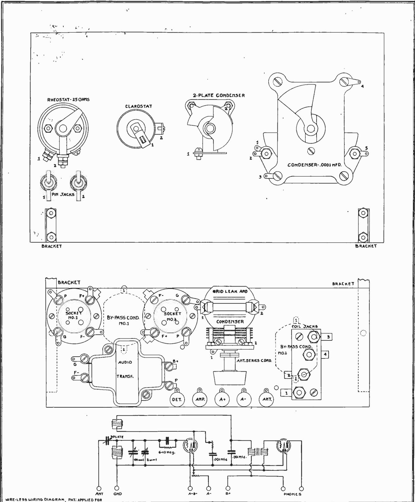
jacent terminals to the left, connect these to the two front plugs inside the coil. You will notice that lugs have been provided for this purpose. The other two plugs are connected to the right hand terminals of the coil.
