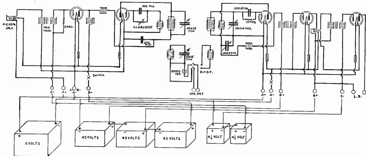
Complete hook-up for B battery operated short wave telephone transmitter and receiver
