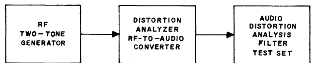
Figure 8-17. Test of Intermodulation in R-F to Audio Converter
