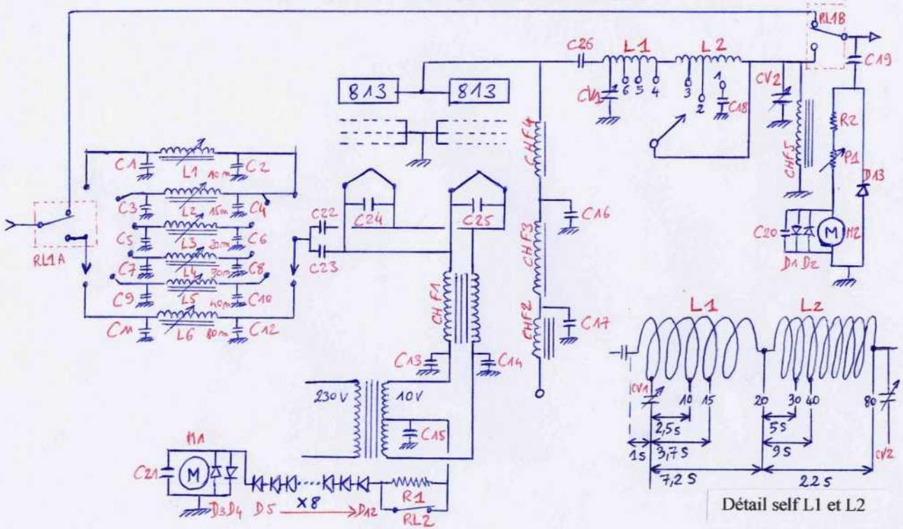
ALIMENTATION HAUTE TENSION, FILAMENT ET 12V
