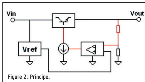
Figure 2: Principe.
