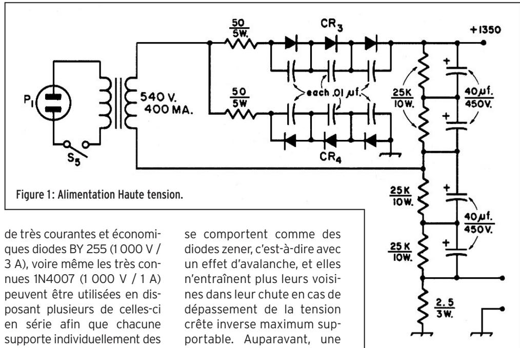
Figure 1: Alimentation Haute tension.
