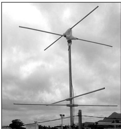
Fig. 7 - Antenne Turnstile (b).
