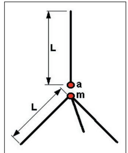
Figure 3 : Antenne "ground-plane".
