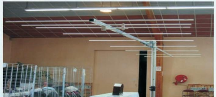
DX.S.R 902 Boom 25x2mm 30x2mm elements 10x1mm
