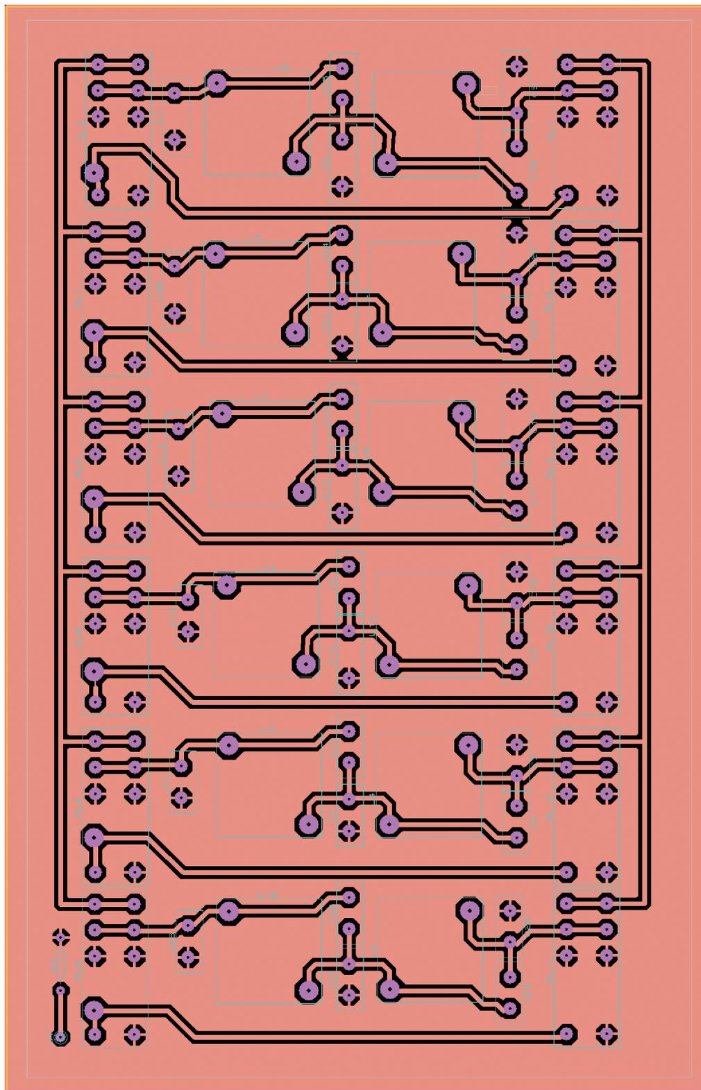
Figure 3 bis: Platine filtres PA: 133 x 207 mm - Implantation.
