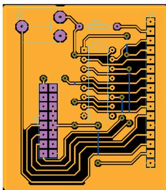
Figure 4 bis: Platine LCD: 42 x 49 mm - Implantation.
