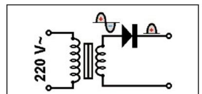
Figure 7 - Redressement mono-alternance.
