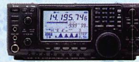
IC-746 E/R TRI-BANDE TOUS MODES 100 W VHF / HF / 50 MHz
