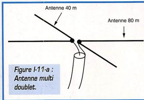
Figure I-11-a : Antenne multi doublet.
