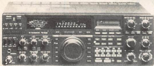
TS 940 SP SSB-AM-FM-FSK 100 KHz-30 MHz-100W HF
