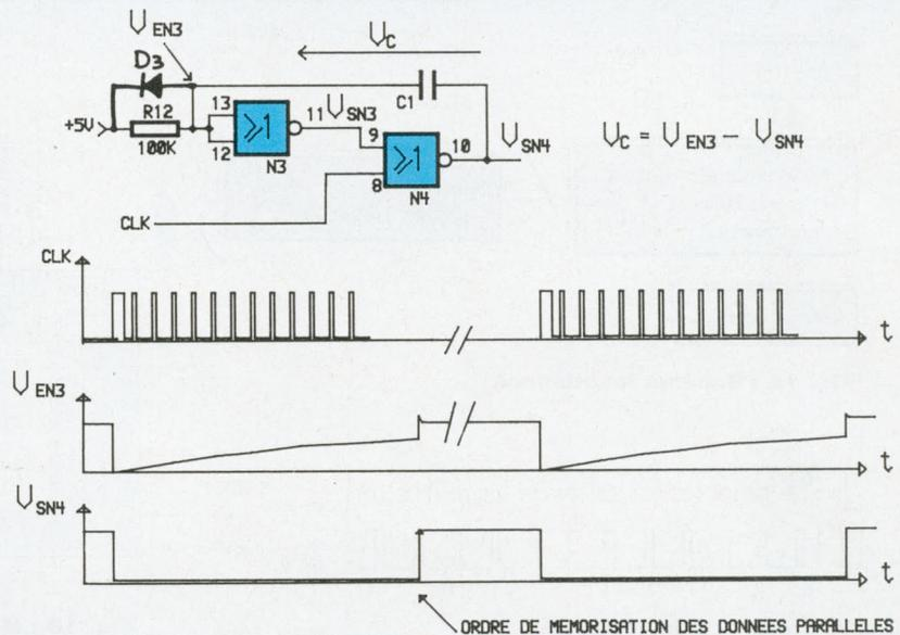
> Au repos  $V_{EN3} = 5$ ,  $V_{SN3} = 0$  V,
