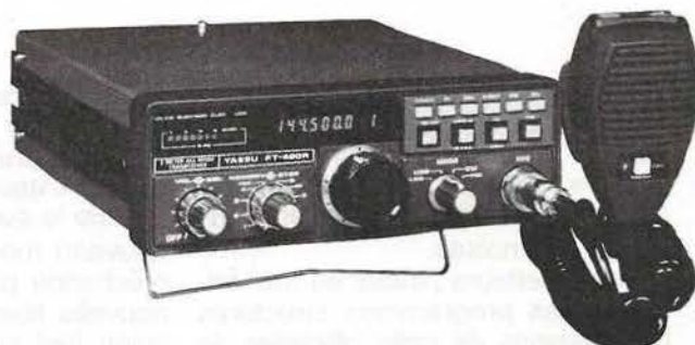
FT 480R Transceiver 144 - 146 MHz, tous modes USB / LSB / FM / CW, 10 W HF, appel 1750 Hz, mémoires programmables, alimentation 12 V.
