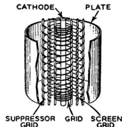
Fig. 37—Structure of remote-cutoff grid.
