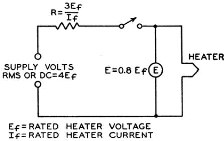
Fig. 124—Test circuit for measuring heater warm-up time.
