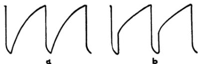
Fig. 91—Waveforms showing effect of  $R_2$  in Fig. 90.
