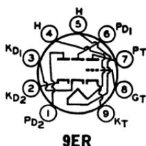
Miniature type used in color and black-and-white television receiver applications. The triode unit is used in burst-amplifier, af amplifier, and low-frequency oscillator applications. The diode units are used in phase-detector, ratio-detector or discriminator, and horizontal afc discriminator circuits. Outlines section, 6E; requires miniature 9-contact socket. Type 8BN8 is identical with type 6BN8 except for heater ratings.
