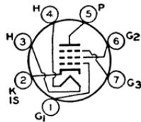
Miniature type used in gated-agc-amplifier circuits and as a noise-inverter tube in color and black-and-white television receivers. Tube has two independent control grids. **Outlines section, 5C**; requires miniature 7-contact socket.
