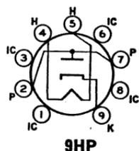
Novar type used as damper tube in horizontal-deflection circuits of color and black-and-white television receivers. Outline section, 30B; requires novar 9-contact socket. Socket terminals 1, 3, 6, and 8 should not be used as tie points. This tube, like other power-handling tubes, should be adequately ventilated.
