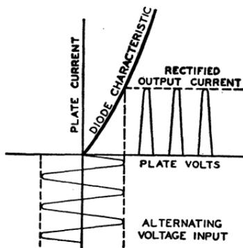
Fig. 4—Current characteristics of rectifier circuit.
