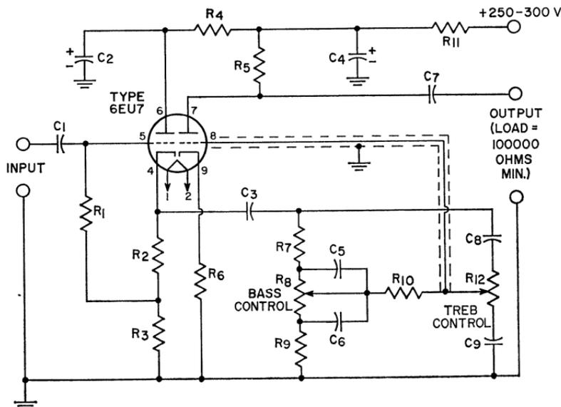
Sensitivity=0.5 volt rms input for output of 1.25 volts with controls set for flat response.
