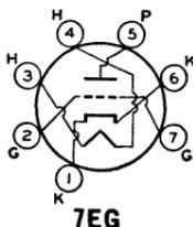
Miniature type used as rf amplifier tube in grid-drive circuits of vhf color and black-and-white television tuners. Outlines section, 5C; requires miniature 7-contact socket. Types 2BN4A and 3BN4A are identical with type 6BN4A except for heater ratings.
