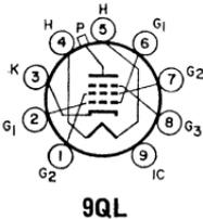
Novar types used as horizontal-deflection amplifier in color and black-and-white television receivers. **Outlines section, 32C**; requires novar 9-contact socket. Types 24LQ6/24JE6C, and 31LQ6 are identical with type 6MJ6/6LQ6/6JE6C except for heater ratings.
