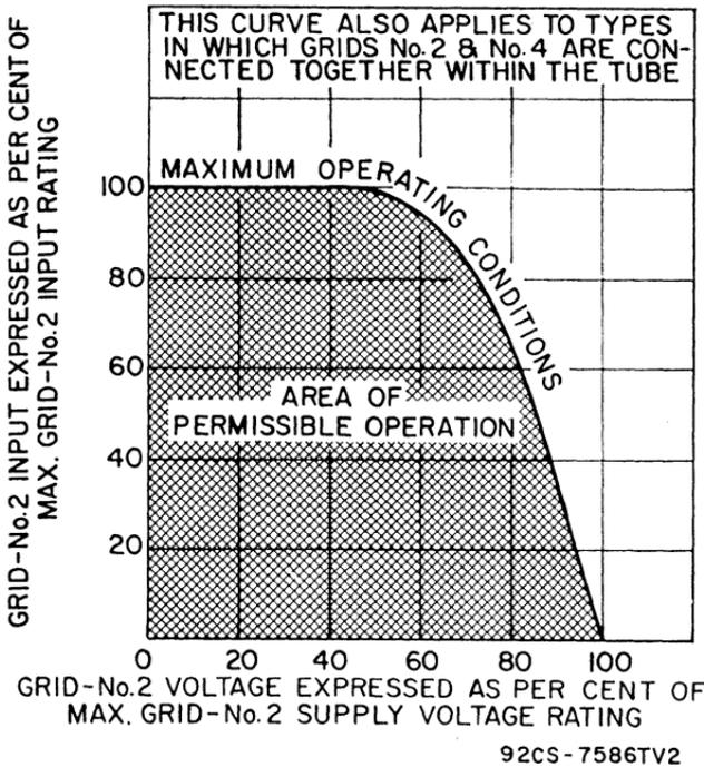
Fig. 134—Grid-No.2 input rating curve.
