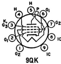
Novar type used in high-efficiency horizontal-deflection-amplifier circuits of television receivers. Outlines section, 18A; requires novar 9-contact socket. For curve of average characteristics see type 6GW6. Types 12GJ5A and 17GJ5A are identical with type 6GJ5A except for heater ratings.
