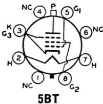
Glass octal type used as horizontal-deflection amplifier in high-efficiency deflection circuits of color and black-and-white television receivers. Outlines section, 21B; requires octal socket. This type may be supplied with pins 1, 4, and 6 omitted. Vertical tube mounting is preferred, but horizontal operation is permissible if pins No.2 and 7 are in vertical plane. Type 25CD6GB is identical with type 6CD6GA except for heater ratings.
