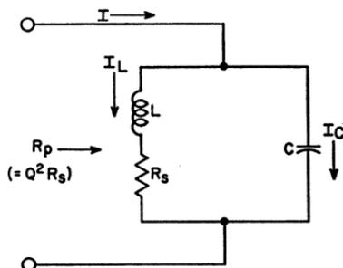
Fig. 67—Simple parallel resonant circuit. (tank) at resonance. The  $Q$  varies inversely with the resistance of the inductor. The lower the resistance, the higher the  $Q$  and the greater the difference between the tank impedance at frequencies off resonance compared to the tank impedance at the resonant frequency.
