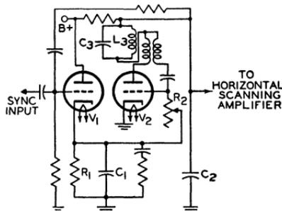
Fig. 101—Simplified synchroguide circuit.
