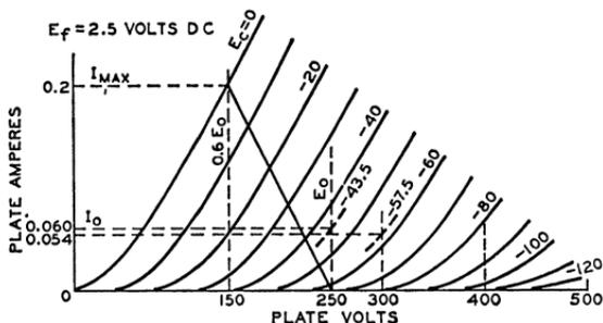
Fig. 42—Graphic calculations for push-pull class A amplifier using a power triode.
