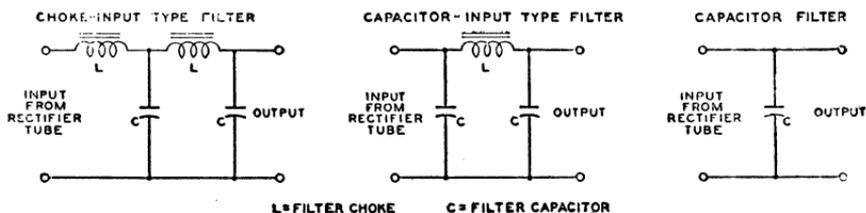
Fig. 121—Typical smoothing filters for rectifier tubes.
