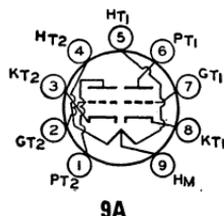
Miniature types used as phase inverters or twin resistance-coupled amplifiers in radio equipment. Outlines section, 6B; require miniature 9-contact socket. Each triode unit is independent of the other except for common heater. For characteristics and curves, refer to type 6AV6. For typical operation as a resistance-coupled amplifier, refer to Resistance-Coupled Amplifier section.
