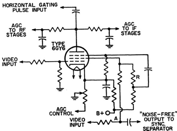
Fig. 84—Typical noise-cancellation circuit.
