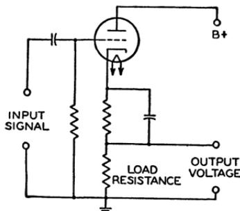
Fig. 52—Cathode-follower circuit modified for increased bias.
