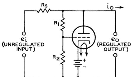
Fig. 92—High-voltage regulator circuit for color television.
