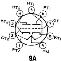
Miniature type used as a phase inverter or push-pull amplifier in mobile communications equipment. **Outlines section, 6B**; requires miniature 9-contact socket. For typical operation as a resistance-coupled amplifier, refer to **Resistance-Coupled Amplifier** section, type 12AU7A conditions.
