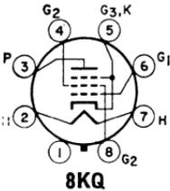
Glass octal type used as audio-frequency power-output tube in high-quality audio applications. **Outlines section, 13D;** requires octal socket. Heater: volts (ac/dc), 6.3; amperes, 0.8; maximum heater-cathode volts,  $\pm 200$  peak, 100 average.
