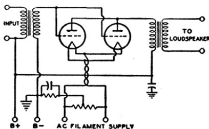
Fig. 39—Power amplifier with tubes connected in parallel.
