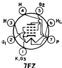
Miniature type used in audio-frequency power-output stage of radio receivers. **Outlines** section, 5D; requires miniature 7-contact socket. The heater is provided with a tap for operation of a panel lamp. **Heater:** volts (ac/dc), 50; amperes, 0.15; tap volts (without panel lamp), 7; maximum heater-cathode volts,  $\pm 200$  peak, 100 average.
