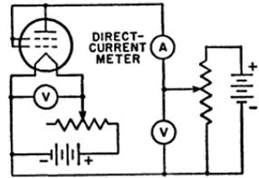
Fig. 129—Fundamental circuit of an emission tester
