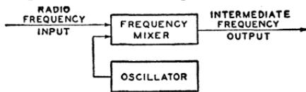
Fig. 106—Block diagram of simple frequency-converter circuit.
