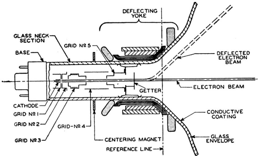
Fig. 10—Structure of television-picture-tube electron gun.
