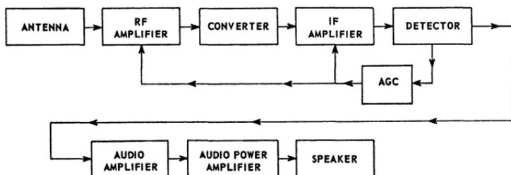
Fig. 14—Simplified block diagram for a broadcast-band receiver.
