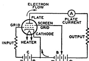
Fig. 7—Basic tetrode circuit.
