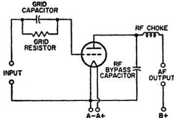
Fig. 27—Detector circuit using grid-resistor-and-capacitor bias.
