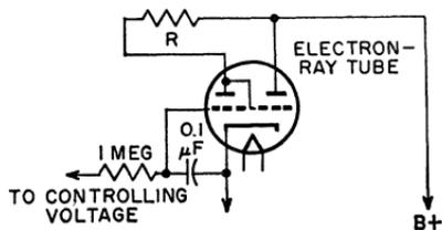
Fig. 110—Indicating circuit using an electron-ray tube.
