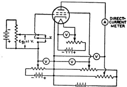
Fig. 130—Fundamental circuit of a transconductance tester using the "grid-shift" method.
