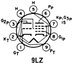
Miniature type used in preamplifier and audio output stages of audio equipment and television receivers. Outlines section, 6G; requires miniature 9-contact socket. **Heater:** volts (ac/dc), 6.3; amperes, 0.7; maximum heater-cathode volts, 100 peak.
