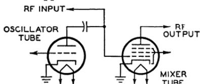
Fig. 108—Typical television mixer-oscillator circuit.
