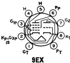
Miniature type used in color and black-and-white television receiver applications. The pentode unit is used as an audio output tube, and the triode unit as an oscillator and af voltage amplifier. Outlines section, 6G; requires miniature 9-contact socket. Type 50BM8/UCL82 is identical with type 6BM8/ECL82 except for heater ratings.
