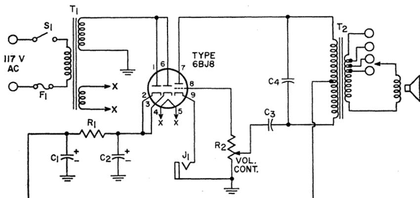
**Note:** Any two terminals of the secondary of  $T_2$  that give the desired tone may be selected. Adjustment of volume control may cause a slight change in tone.
