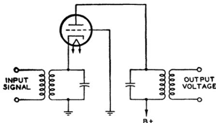
Fig. 47—Cathode-drive circuit.
