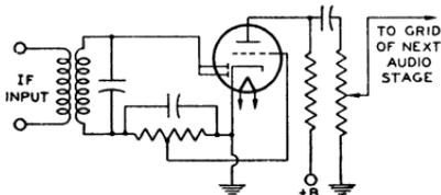
Fig. 25—Diode-biased detector circuit.
