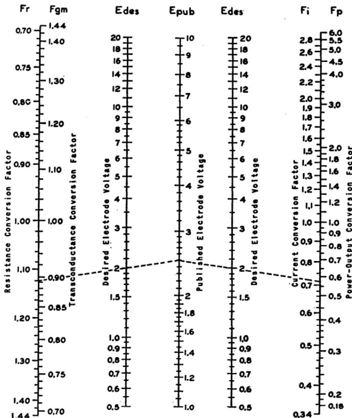
Fig. 44—Nomograph of tube conversion factors.
