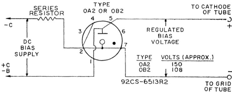
Typical circuit for bias-supply regulation. Removal of tube from socket opens B-supply circuit of regulated tubes.
