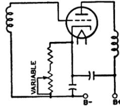
Fig. 115—Amplifier stage similar to Fig. 114 but using heater-cathode-type tube.
