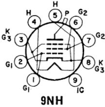
Magnoval type used as horizontal-deflection amplifier in television receivers. **Outlines section, 35B**; requires neonval 9-contact socket. Typical instantaneous characteristics (measured with recurrent waveform such that maximum ratings are not exceeded): plate volts, 75; grid-No.2 volts, 200; grid-No.1 volts, -10; plate mA, 440; grid-No.2 mA, 37. Types 13GB5/XL500, 18GB5/LL500 and 27GB5/PL500 are identical with type 6GB5/EL500 except for heater ratings.
