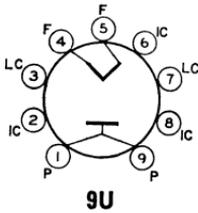
Miniature type used as a high-voltage, low-current pulse-operated focus rectifier in color television receivers. The filament of the tube can be operated directly across the filament winding of the horizontal-output transformer without a series voltage-dropping resistor. Outlines section, 6B; requires miniature 9-contact socket.
