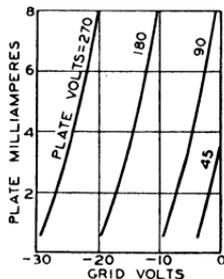
Fig. 13—Family of transfer-characteristic curves.
