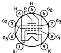
Magnoval type used as a horizontal-deflection amplifier in color television receivers. Outlines section, 38A; requires 9-contact magnoval socket. Type 40KG6A/PL509 is identical with type 6KG6A/EL509 except for heater ratings.
