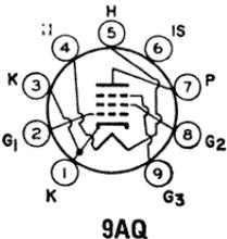
Miniature types used as if-amplifier tubes in color and black-and-white television receivers. Outlines section, 6C; requires miniature 9-contact socket. Types 3EJ7/XF184 and 4EJ7/LF184 are identical with type 6EJ7/EF184 except for heater ratings.
