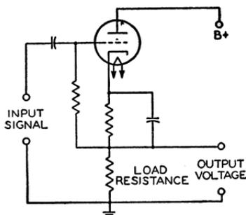
Fig. 53—Cathode-follower circuit modified for reduced bias.
