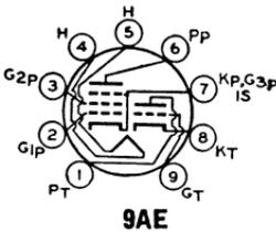
Miniature types used as combined oscillator and mixer tube in color and black-and-white television receivers utilizing an intermediate frequency in the order of 40 MHz. Outlines section, 6B; require miniature 9-contact socket. Type 5U8 is identical with type 6U8A/6KD8 except for heater ratings.
