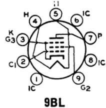
Miniature type used as power amplifier tube in high-fidelity audio equipment. Outlines section, 6G; requires miniature 9-contact socket.
