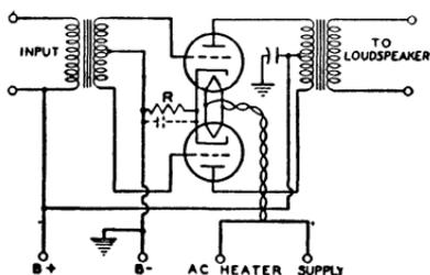
Fig. 40—Power amplifier with tubes connected in push-pull.
