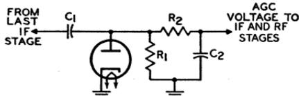
Fig. 63—Automatic-gain control (agc) circuit.
