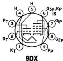
Miniature type used in television receiver applications. The triode unit is used as a general-purpose amplifier; the pentode unit is used as a video amplifier. Outlines section, 6E; requires miniature 9-contact socket. Type 10KR8 is identical with type 6KR8 except for heater ratings.
