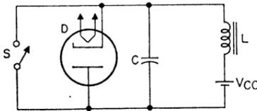
Fig. 88—Incorporation of damper diode.
