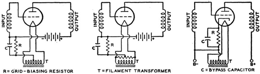
Fig. 113—Typical grid-voltage supply circuits.
