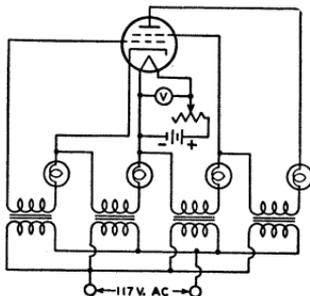
Fig. 128—Fundamental circuit of a short circuit tester.
