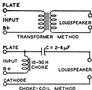
Fig. 123—Typical output-coupling devices.
