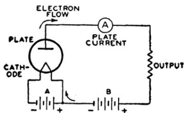
Fig. 3—Basic diode circuit.
