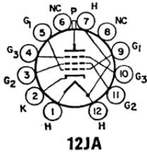
Duodec type used as a horizontal-deflection amplifier in color and black-and-white television receivers. **Out-lines section, 16C**; requires duodec 12-contact socket. **Heater:** volts (ac/dc), 26; ampere, 0.6; warm-up time, 11 seconds; maximum heater-cathode volts,  $\pm 200$  peak, 100 average.
