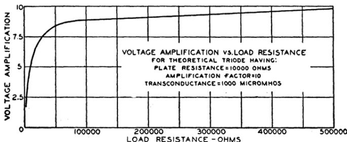
Fig. 36—Gain curve for triode amplifier circuit.
