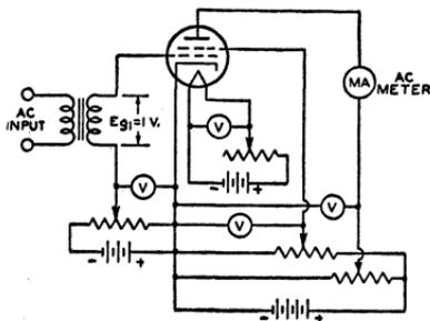
Fig. 131—Fundamental circuit of a dynamic transconductance tester.
