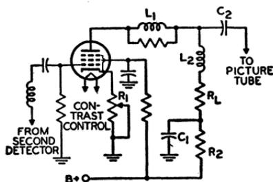
Fig. 76—Typical video amplifier stage.
