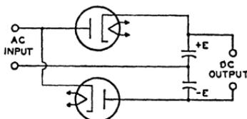
Fig. 19—Full-wave voltage-doubler circuit.
