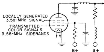
Fig. 97—Low-level color demodulator.
