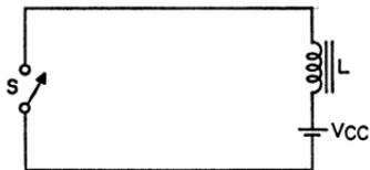
Fig. 85—Simplest form of deflection circuit.
