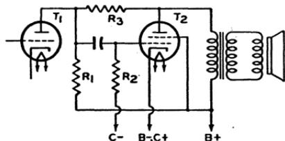
Fig. 50—Resistance-coupled stages using feedback resistor.
