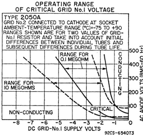
The shield grid (grid No. 2) is normally connected to the cathode at socket. It may, however, be used as a control electrode because the control characteristic of grid No. 1 may be shifted by varying the potential of grid
