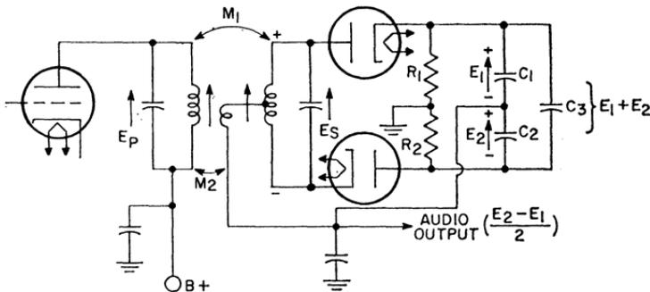
Fig. 33—Ratio-detector circuit.
