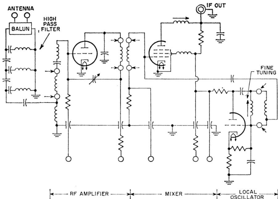
Fig. 72—Simplified schematic of typical vhf television tuner.
