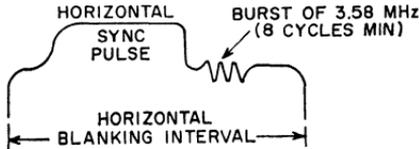
Fig. 96—Waveform for synchronizing signal.
