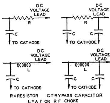
Fig. 120—Typical filter circuits.
