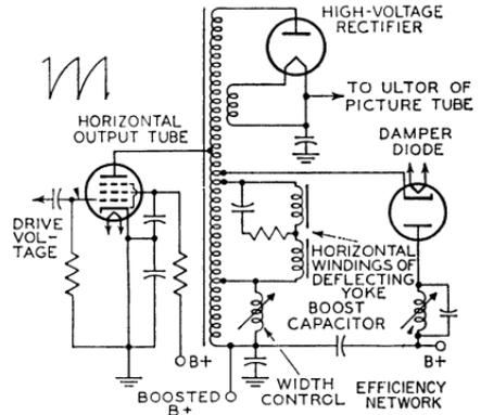
Fig. 89—Typical horizontal-deflection and high-voltage circuit.
