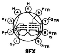
Miniature type used as combined vhf oscillator and mixer in color and black-and-white television receivers. Outlines section, 6B; requires miniature 9-contact socket. For maximum ratings as class A<sub>1</sub> amplifier, see type 6U8A. Type 5CL8A is identical with type 6CL8A except for heater ratings.
