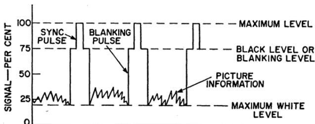
Fig. 79—Detected video signal.
