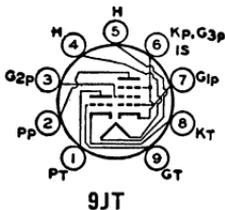
Miniature type used in high-quality, high-fidelity audio equipment, particularly in phase splitters, tone-control amplifiers, and high-gain voltage amplifiers. **Outlines** section, 6B; requires miniature 9-contact socket. For operation as resistance-coupled amplifier, refer to **Resistance-Coupled Amplifier** section. In direct-coupled voltage-amplifier phase-splitter circuits, the pentode unit should drive the triode unit.
