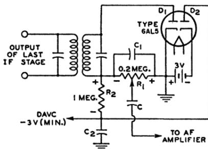
Fig. 62—Delayed avc (davc) circuit.
