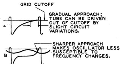
Fig. 103—Waveforms showing effect of tuned circuit L<sub>3</sub>C<sub>3</sub> in Fig. 101.
