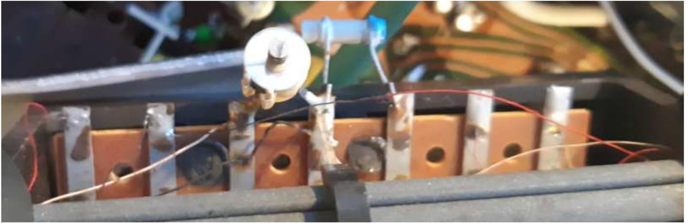
Raccordement antenne ferrite
