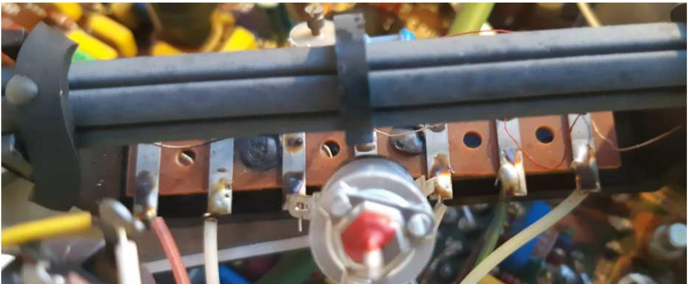
Raccordement antenne ferrite
