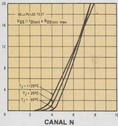
Figure 5 - Courbes  $I_O = f(V_{GS})_{T=cte}$
