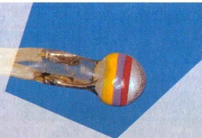
**UNE CTN BRANCHÉE AU BOUT D'UN CABLE BIFILAIRE.**
