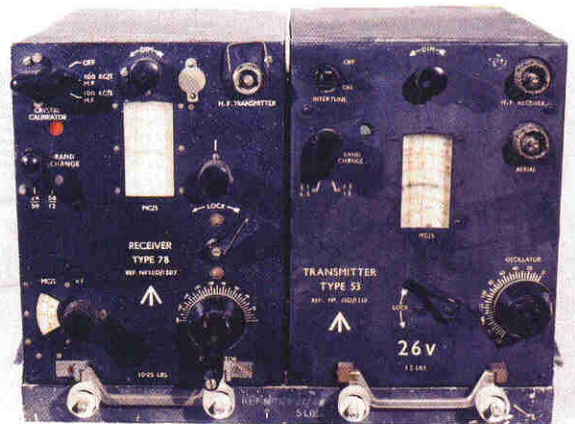
Fig. 1: The Receiver 78 and Transmitter 53 in a mounting cradle.
