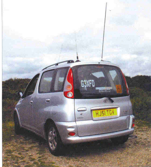
Fig. 1: Rear view of the G3XFD 'travelling Amateur Radio station', showing the 144MHz whip (left) and the 7MHz Pro-AM h.f. whip (removed when travelling). The Toyota Yaris MPV is equipped for h.f. and v.h.f. operations. The internal lay-out of vehicle provides many 'nooks and crannies' for stowing equipment. The Yaris is fitted with air conditioning and is also provided with picnicking and tea & coffee making facilities (Well he does spend a lot of time driving!). And yes, the 'TGV' of the number plate was especially chosen...even though he doesn't try to race real TGV trains when in France! (See text).
