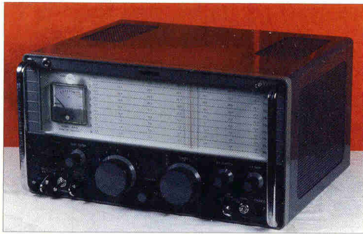
● It's A Classic! The Eddystone EA12 receiver. The small control above the S-meter is the calibrator On-Off push button. The knurled spindle on the right hand opposite side, is the cursor adjustment for calibration purposes (see text). Photographic facilities courtesy of Ken O'Brien.
