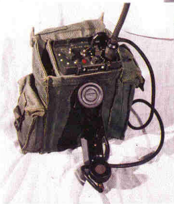
● Fig. 4: The CPRC-26 in canvas case with handset and whip antenna (See text).
