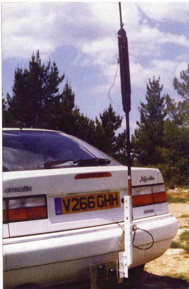
● Fig. 5: Full end-on view of MOEJB's car with the Midge Catcher in place and operational. Note the flying leads for selecting tapping points. See text for mounting and attachment suggestions.
