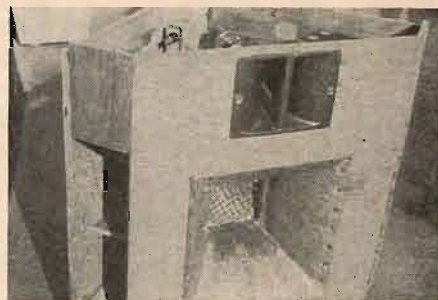
Fig. 9. Method of mounting horns to front of cabinet structure.
