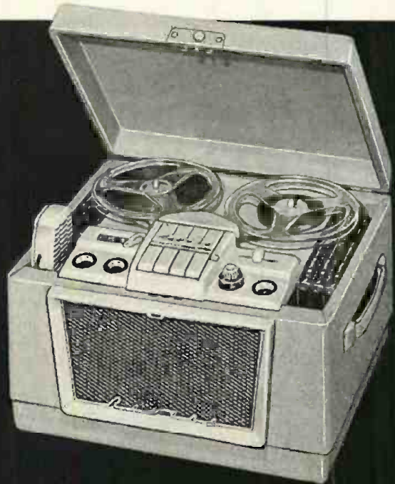
T-700-D DUAL-SPEED DELUXE. Records up to 3 hours with long-play tape. Automatic keyboard controls; index counter. FREQ. RESPONSE: 3.75 i.p.s.—40-7,500 ± 3DB; 7.5 i.p.s. 40-14,500 ± 3DB. WOW 0.3% Max. With microphone, radio attach. cord, tape, reels, $212.50
