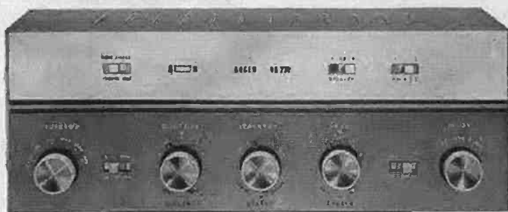
DB 230. STEREO CONTROL CENTER AND DUAL 30-WATT AMPLIFIER.
