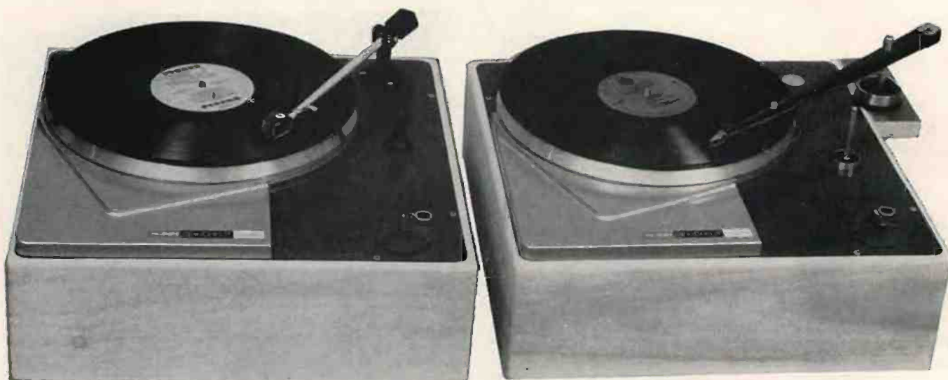
MOUNTED ON MATCHED Rek-O-Kut N-33H single speed turntables were the Scott-London Type 1000 (left) and Shure Studio Dynetic (right) arms.
