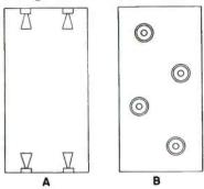
Fig. 12. Two possible horn locations in a factory building 50 x 100 feet. A—straight reentrant horn-type speaker.
