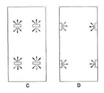
Fig. 11. Four possible speaker placements in an office 50 x 190 feet. A & C—cone speakers in two-way baffles. B & D—cone speakers in wall mounting baffles.
