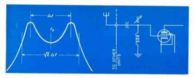
Fig. 2 (left). Curve resulting from over-coupled circuits of Fig. 1. The usable band width is represented by the limits  $\sqrt{2} \Delta f$ . The valley between the peaks can be filled by using a single-tuned circuit in conjunction with the doubletuned circuits. Fig. 3 (right). Method of coupling the antenna to each of the tuner strips. This enables tuning the antenna circuit for each station and provides adequate signal input to the first stage.
