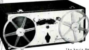
The basic Magnecorder recorder mechanism (PT6-A)
