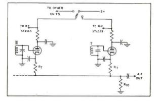
In order to reduce the effect of the valley between the two peaks, a single tuned circuit is employed for the antenna coupling, as shown in Fig. 3. The coils used have adjustable cores, and the tuning capacitances are fixed. Since a number of tuners are to remain connected to the antenna at all times, the coupling to the antenna is such as to load the circuit only at the frequency of operation, rather than throughout the entire band. Thus a
