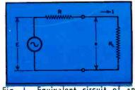
Fig. 1. Equivalent circuit of an amplifier.
