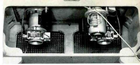
Fig. 4. Capstan drive includes resilient coupling, above motor, and crankactuated idler which presses tape against driving shaft, above top plate. Assembly is adjustable for tape alignment.
