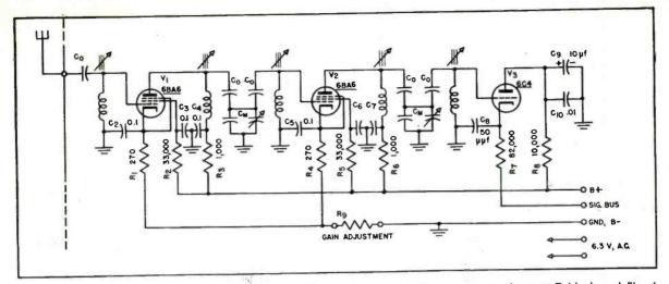
Fig. 5. Over-all schematic for the AM tuner strip. Values for Co and Cx are given in the text. Table I, and Fig. 6.
