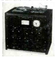
Five input channels accommodate three microphones, one phono pickup or telephone line, and a radio tuner. Individual adjustments are provided for the supersonic frequency bias and erase voltages. The supersonic bias frequency range is adjustable from 30 to 80 kc. Total recording and playback distortion at 400 cycles is under 3%.
