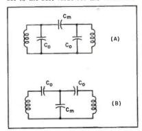
Fig. 1. Two methods of obtaining band-pass coupling by the use of two tuned circuits and an impedance common fo both. (A). High-impedance capacitance coupling; (B). Low-impedance capacitance coupling
