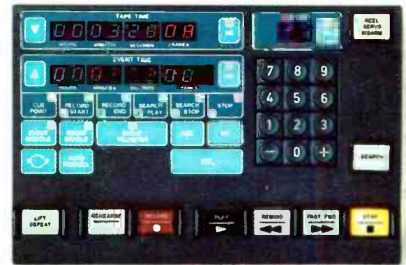
ATR-124's Multi-Point Search-To-Cue (MPSTC). Provides 100 cue locations.
