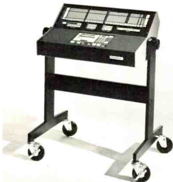
Figure 2. A roll-around pedestal containing the channel function and multi-point search-to-cue modules.
