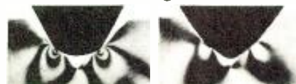
Stress analysis photos show concentrated high pressure with elliptical stylus (left), reduced pressure, less groove distortion with Shibata stylus (right).
