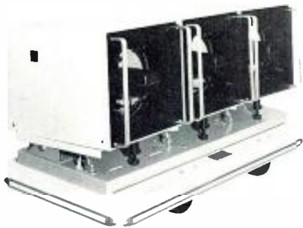
Figure 2. The three heads of the Image Magnification large-screen projector. The entire unit can be operated remotely from up to 100 feet away. A detail enhancer is built in.
