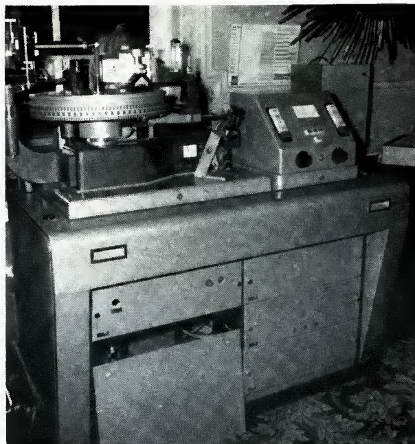
Figure 6. Crowds formed around demonstrations (as they have done in the U.S.) of the Neumann computer-controlled disc mastering lathe, model VMS 66.
