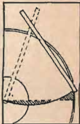
How Conventional Tone Arms Create Tracking Error (See Shaded Area).
