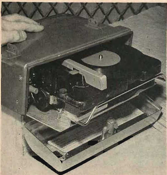
Fig. 3. The Highway Hi-Fi record player removed from its underdash mounting. Note reversed pickup arm.
