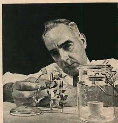
Through the study of thousands of specially cultivated whiskers, Bell scientists seek to prevent treacherous growths in telephone equipment.
