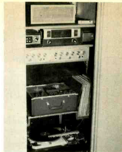
Fig. 5—The author's present system includes the following components: ADC 10E stereo cartridge in a special moving-pivot tone arm; Thoren TD-124 manual turntable; Ampex 1260 4-track tape recorder; Marantz mono preamplifiers; Knight AM tuner; Fisher FM tuner; Marantz electronic crossovers at 100 Hz and 3500 Hz; JBL N-500 crossover networks at 500 Hz; Eico 28-watt dual basic amplifier above 3500 Hz; Marantz 40-watt basic amplifiers between 100 Hz and 3500 Hz. The latter drives JBL theatre woofers to 500 Hz and Stephens P-35 theatre drivers above 500 Hz. A Marantz 40-watt basic amplifier drives an Electro-Voice 15-in. "K" horn; Ionovac tweeters and JBL high-frequency lenses round out the system.
