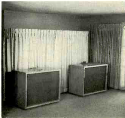
Fig. 4—Since it was impossible to conceal the big horns fully without making the listening room seem about 1/3rd smaller, draperies were placed 2 1/2 ft. back.
