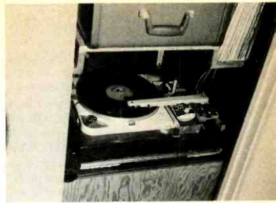
Fig. 1—To minimize lateral and vertical pivot friction, the author's moving-pivot tone arm floats on distilled water.
