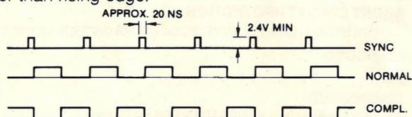
**Square Wave Mode.** Automatically sums pulse width and pulse spacing, converting the output to a symmetrical square wave with a period equal to twice their sum.
