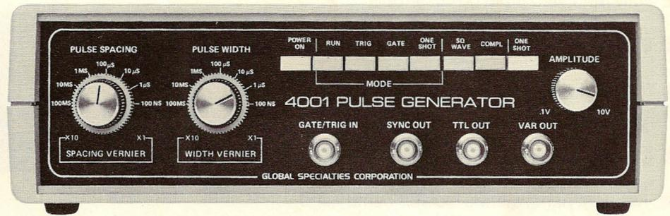
The Model 4001 Ultravariabe Pulse Generator™ is uniquely designed to permit precise tailoring of pulse repetition rate and duty cycle over a wide range through the independent setting of pulse spacing and pulse width. Both pulse width and pulse spacing are continuously variable over seven decade ranges from 100 ns to 1 s, outputs from 0.5 Hz to 5.0 MHz.
