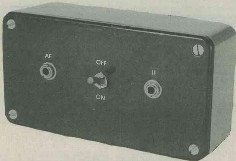
The test oscillator can be housed in any small plastic case which can accommodate the components
