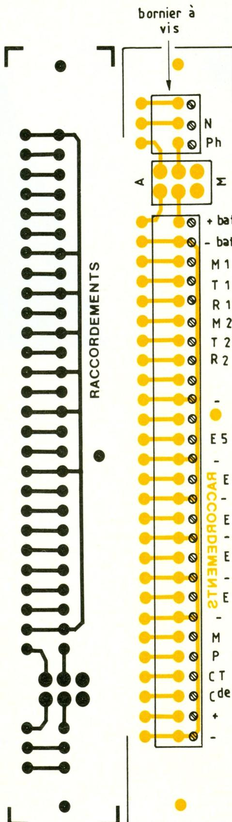
Photo 5. - Le BUS de raccordement.
