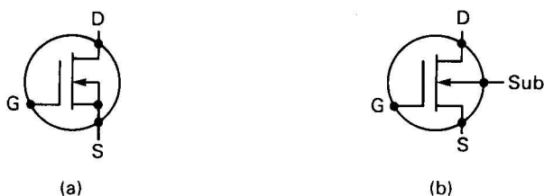
Figure 10.1 Standard symbols of (a) three-pin and (b) four-pin n-channel depletion-mode MOSFETs
