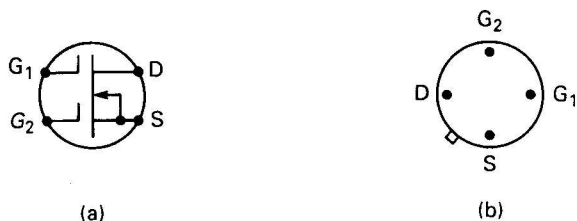
Figure 10.2 Symbol (a) and TO72 outline (b) of the 3N140 and 40673 dual-gate or 'tetrode' MOSFET
