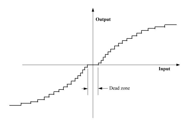
FIGURE 3.4 Non-linear quantizer characteristic
