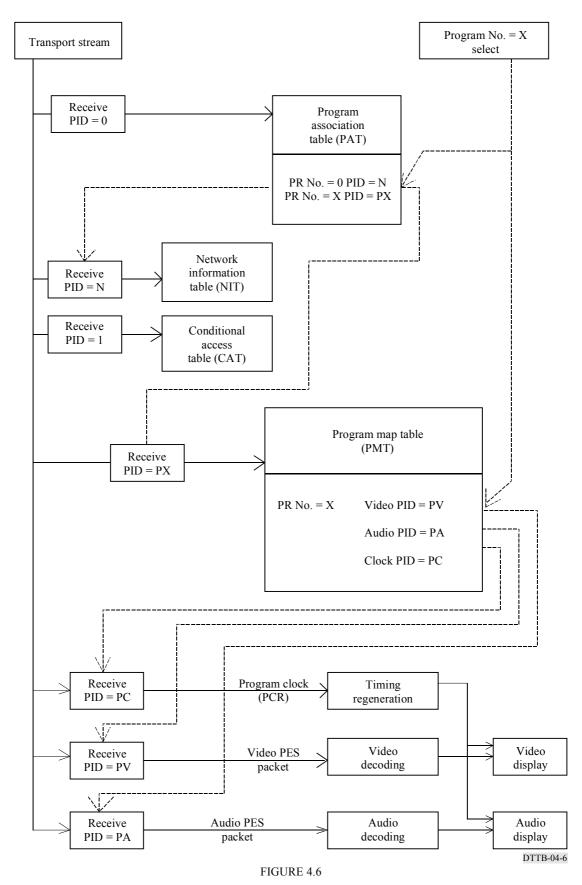
An example of data access flow in the receiver
