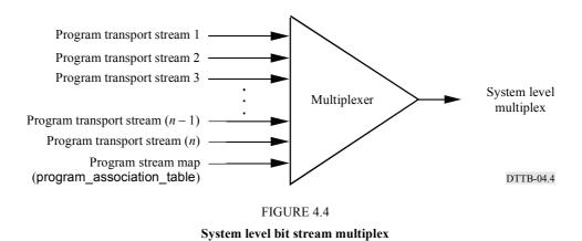
This process can be made scalable by multiplexing multiple system level bit streams on a higher bandwidth channel by extracting the program\_association\_tables from each system multiplexed bit stream and reconstructing a new PID = 0 bit stream.
