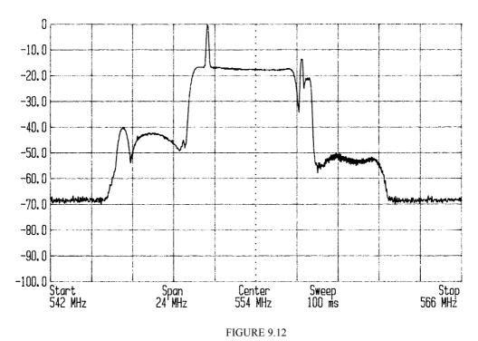
Spectrum for a system G 40 kW pulsed klystron transmitter with FM-sound and NICAM carriers
