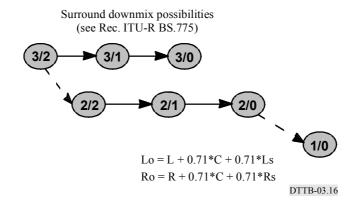
Down mix from 3/2 down to 1/0 for a future multichannel audio system
