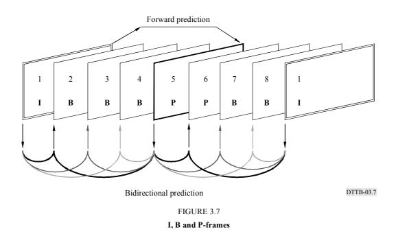
The predicted frame (5) is derived from the intra-frame (1) initially sent, i.e. frame (1) becomes the "previous frame" and frame (5) the "current frame" in the description contained in § 3.5.4.
