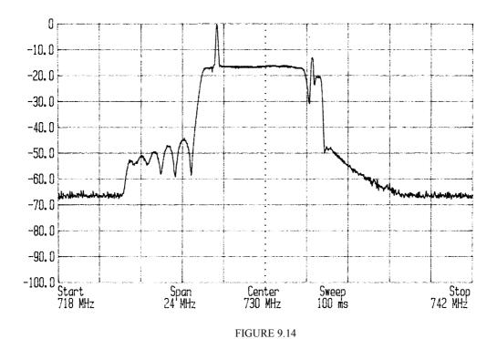
Spectrum for a system G 10 kW tetrode transmitter with FM-sound and NICAM carriers
