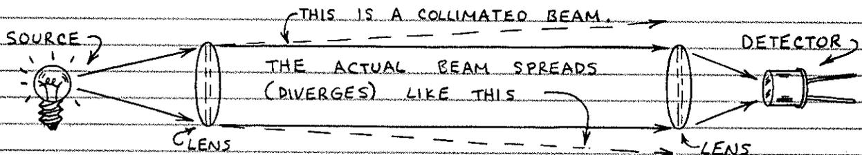
THE BEAM SPREAD ANGLE (THE DIVERGENCE) IN RADIANS\* IS THE DIAMETER OF THE SOURCE DIVIDED BY THE FOCAL LENGTH OF THE LENS. THIS MEANS LENSES WITH LONGER FOCAL LENGTHS GIVE NARROWER BEAMS. (BUT LENSES WITH LONG FOCAL LENGTHS COLLECT LESS LIGHT THAN THOSE WITH SHORT FOCAL LENGTHS...)
