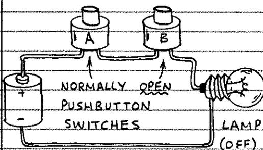
THE LAMP GLOWS ONLY WHEN SWITCHES A AND B ARE CLOSED. THE TABLE SUMMARIZES THE GATE'S OPERATION. IT'S CALLED A TRUTH TABLE.
