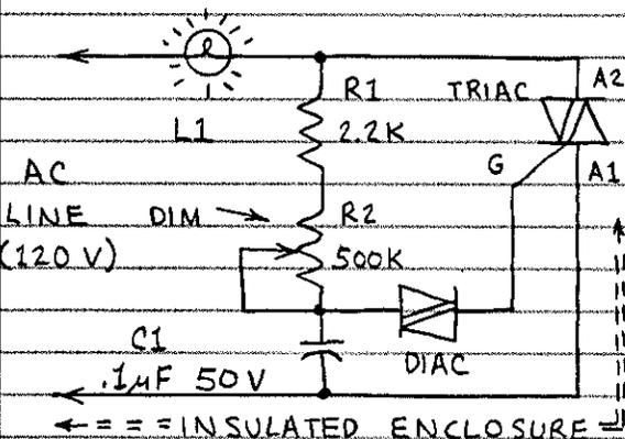
THIS IS HOW MANY HOUSEHOLD DIMMER SWITCHES ARE MADE. L1 CAN BE UP TO 100 WATT (120 VOLT) LAMP. USE HEAT SINK ON TRIAC IF IT BECOMES HOT. THE DIAC IS A BIDIRECTIONAL TRIGGER DIODE. CAUTION: THIS CIRCUIT MUST BE FULLY ENCLOSED AT ALL TIMES WHEN POWER IS APPLIED!
