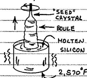
SILICON CAN BE GROWN INTO BIG CRYSTALS. IT'S CUT INTO WAFERS FOR MAKING ELECTRONIC PARTS.
