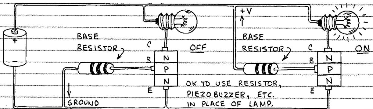
ONLY TWO INPUTS ARE POSSIBLE: GROUND (0 VOLTS) AND THE POSITIVE BATTERY VOLTAGE (+V). THEREFORE THE TRANSISTOR IS OFF OR ON. A TYPICAL BASE RESISTANCE IS 5,000 TO 10,000 OHMS. (IF THE RESISTOR IS REPLACED BY A WIRE, THE LAMP CAN BE SWITCHED ON OR OFF FROM A CONSIDERABLE DISTANCE.)
