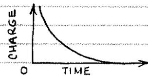
□ SPECIFYING CAPACITORS — THE ABILITY TO STORE ELECTRONS IS KNOWN AS CAPACITANCE. CAPACITANCE IS SPECIFIED IN FARADS. A 1-FARAD CAPACITOR CONNECTED TO A 1-VOLT SUPPLY WILL STORE 6,280,000,000,000,000,000 ( $6.28 \times 10^{18}$ ) ELECTRONS! MOST CAPACITORS HAVE MUCH SMALLER VALUES. SMALL CAPACITORS ARE SPECIFIED IN PICOFARADS (TRILLIONTHS OF A FARAD) AND LARGER CAPACITORS ARE SPECIFIED IN MICROFARADS (MILLIONTHS OF A FARAD). SUMMING UP:
