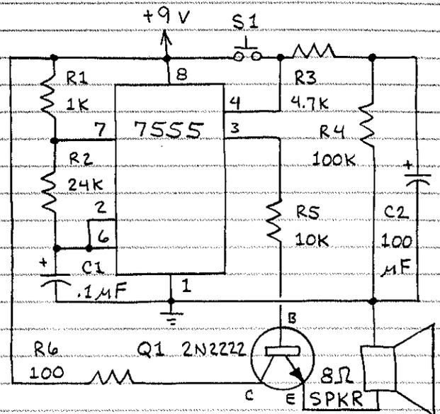
PRESS S1 AND THE SPEAKER EMITS A TONE. RELEASE S1 AND THE TONE CONTINUES FOR SEVERAL SECONDS. C2 AND R4 CONTROL DELAY. C1 CONTROLS FREQUENCY. (USE 7555 ONLY. 555 USES TOO MUCH CURRENT.)
