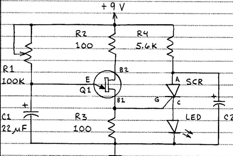
WHEN THE SCR IS OFF, C2 CHARGES THROUGH R4. WHEN THE SCR IS TURNED ON BY A PULSE FROM UJT Q1, THE CHARGE IN C1 IS RAPIDLY "DUMPED" THROUGH THE LED. THE SCR (AND LED) THEN TURNS OFF SINCE THERE IS NO LONGER SUFFICIENT HOLDING CURRENT. THE CYCLE THEN REPEATS.
