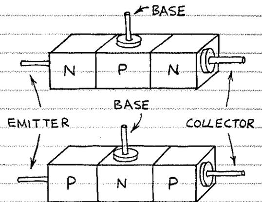
□ BIPOLAR TRANSISTOR OPERATION — THE THREE LAYERS OF A BIPOLAR TRANSISTOR ARE THE EMITTER, BASE AND COLLECTOR. THE BASE IS VERY THIN AND HAS FEWER DOPING ATOMS THAN THE EMITTER AND COLLECTOR. THEREFORE A VERY SMALL EMITTER — BASE CURRENT WILL CAUSE A MUCH LARGER EMITTER — COLLECTOR CURRENT TO FLOW.
