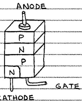
□ SCR OPERATION — IF THE ANODE OF AN SCR IS MADE MORE POSITIVE THAN THE CATHODE THE TWO OUTERMOST PN JUNCTIONS ARE FORWARD BIASED.
