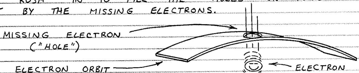
□ MISSING ELECTRONS — MECHANICAL FRICTION, LIGHT, HEAT OR A CHEMICAL REACTION MAY REMOVE ELECTRONS FROM A SURFACE. THIS CAUSES THE SURFACE TO BE POSITIVELY CHARGED. SINCE THE POSITIVELY CHARGED ATOMS ARE AT REST, THE SURFACE CAN BE SAID TO HAVE A POSITIVE STATIC ELECTRICAL CHARGE.
