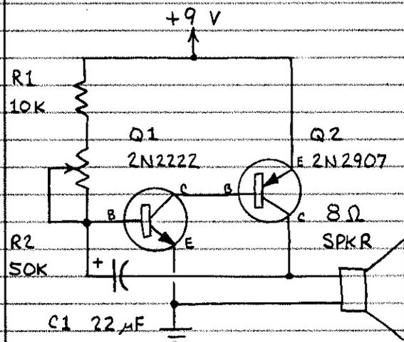
A METRONOME MARKS TIME BY PRODUCING A REGULAR SEQUENCE OF "CLICKS" OR "POCKS." ADJUST THE CLICK RATE BY ADJUSTING R2 OR CHANGING C1'S VALUE.
