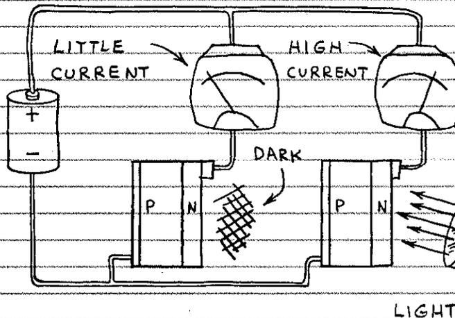
2. PHOTOCONDUCTIVE OPERATION - HERE THE PHOTODIODE IS REVERSE-BIASED. A CURRENT FLOWS WHEN THE PN JUNCTION IS ILLUMINATED. (WHEN DARK, A TINY CURRENT CALLED THE DARK CURRENT WILL FLOW.)
