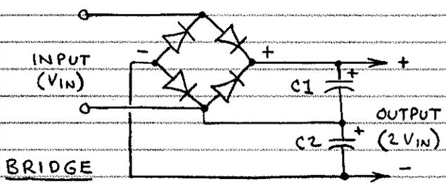
THE BRIDGE DOUBLER IS MORE EFFICIENT THAN THE CONVENTIONAL AND CASCADE DOUBLERS. SINCE 4-DIODE BRIDGE RECTIFIERS ARE AVAILABLE, IT'S EASY TO MAKE.
