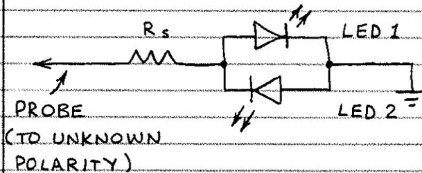
THIS CIRCUIT INDICATES THE POLARITY OF A VOLTAGE.  $R_s$  MUST BE USED (SEE ABOVE).
