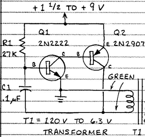
THIS CIRCUIT PRODUCES 220 VOLT PULSES OF DC WHEN POWERED BY A 9-VOLT BATTERY. IT WILL PRODUCE UP TO 170 VOLTS FROM A FLASHLIGHT CELL (BUT YOU MAY HAVE TO EXPERIMENT WITH C1'S VALUE. THE CIRCUIT WILL POWER ONE OR MORE NEON LAMPS THROUGH A 1M SERIES RESISTOR.
