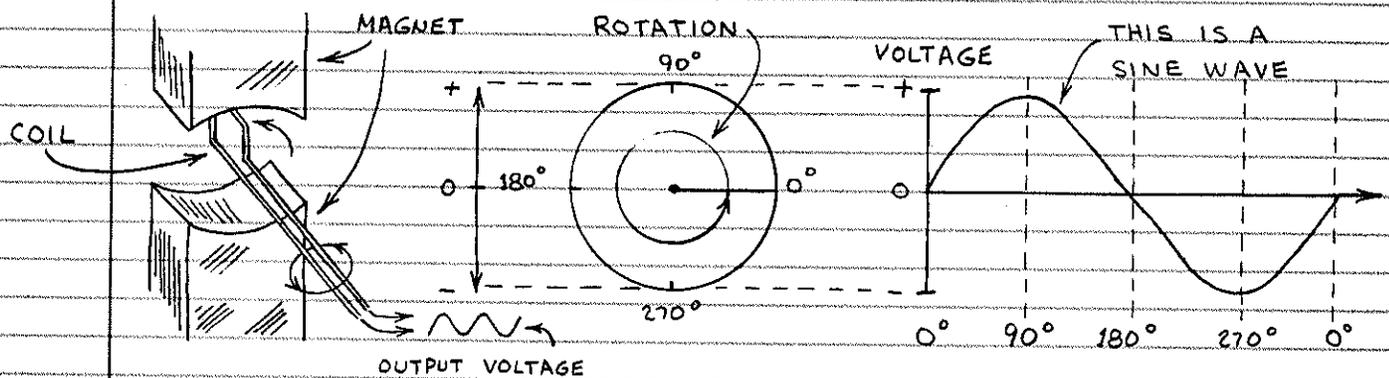
ROTATING COIL      VOLTAGE OUTPUT      AC SINE WAVE
