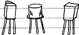
SMALL SIGNAL TRANSISTORS ARE USED TO AMPLIFY LOW LEVEL SIGNALS. SWITCHING TRANSISTORS ARE DESIGNED TO BE OPERATED FULLY ON OR OFF. SOME TRANSISTORS CAN BOTH AMPLIFY AND SWITCH EQUALLY WELL.
