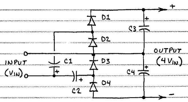
TRIPLES AND CONVERTS TO DC AN INCOMING AC VOLTAGE. C2, D1, D2 AND D3 RATED AT  $>2V_{IN}$ .
