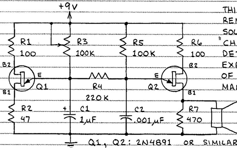
THIS CIRCUIT PRODUCES A REMARKABLE VARIETY OF SOUNDS. AS SHOWN, IT "CHIRPS" AT A RATE DETERMINED BY R3. EXPERIMENT WITH VALUES OF C1, R5 AND C2 FOR MANY OTHER EFFECTS.
