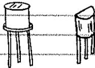
MOST LASCRs CAN SWITCH UP TO A FEW HUNDRED VOLTS. MAXIMUM CURRENT IS ONLY A FEW TENTHS OF AN AMPERE.
