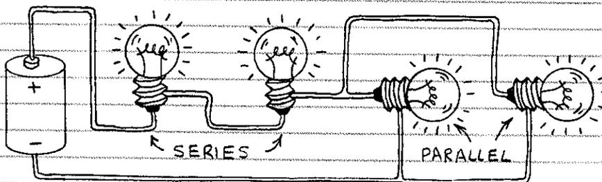
MANY ELECTRICAL CIRCUITS ARE BOTH SERIES AND PARALLEL. ALL PROVIDE A COMPLETE PATH BETWEEN THE CIRCUIT AND ITS POWER SUPPLY.
