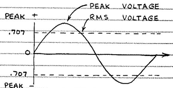
□ WHY AC IS USED - AC IS BETTER SUITED THAN DC FOR TRANSMISSION THROUGH LONG DISTANCE POWER LINES. A WIRE CARRYING AC WILL INDUCE A CURRENT IN A NEARBY WIRE. THIS IS THE PRINCIPLE BEHIND THE TRANSFORMER.
