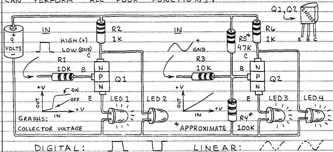
HERE TRANSISTOR Q1 IS USED AS A SWITCH. WHEN THE INPUT IS NEAR +V (OR HIGH), Q1 TURNS ON AND LED1 IS ILLUMINATED. WHEN THE INPUT IS NEAR GROUND (OR LOW), Q1 TURNS OFF. THIS TURNS LED 1 OFF AND ALLOWS LED 2 TO GLOW. (R2 CONTROLS THE CURRENT THROUGH BOTH LEDs.) THIS CIRCUIT IS THEN A COMBINED DIGITAL BUFFER AND INVERTER.
