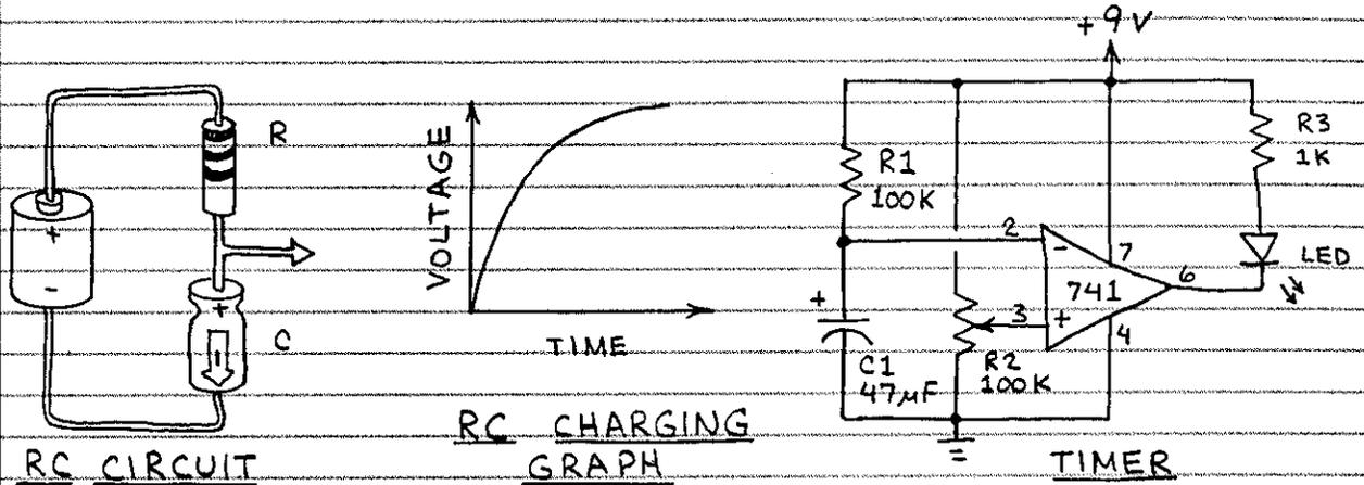
IN THE CIRCUIT DIAGRAM (ABOVE RIGHT), R1 AND C1 FORM AN RC CIRCUIT. C1 GRADUALLY CHARGES TO +9 VOLTS THROUGH R1. WHEN THE VOLTAGE ON C1 EXCEEDS THE REFERENCE VOLTAGE SUPPLIED TO THE NON-INVERTING INPUT OF THE OP-AMP, ITS OUTPUT SWINGS FROM HIGH TO LOW AND THE LED GLOWS. THE TIME DELAY CAN BE CHANGED BY ALTERING THE VALUES OF R1 AND C1 OR THE SETTING OF R2. DISCHARGE C1 (USE PUSHBUTTON SWITCH) FOR NEW CYCLE.
