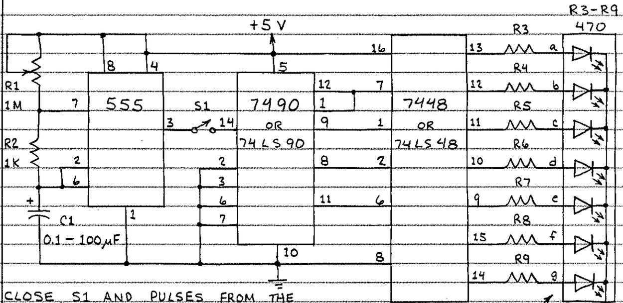
CLOSE S1 AND PULSES FROM THE 555 WILL BE COUNTED BY THE 7490. THE 7448 CONVERTS THE BCD OUTPUT FROM THE 7490 INTO 7-SEGMENT DIGITS ON AN LED DISPLAY. ADJUST R1 AND C1 FOR DESIRED PULSE RATE. TO ADD ADDITIONAL DIGIT:
