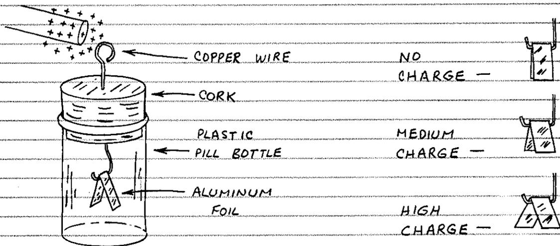
BE SURE THE FOLDED FOIL STRIP IS CLEAN AND DRY. WHEN YOU TOUCH A CHARGED OBJECT TO THE WIRE, THE TWO HALVES OF THE FOIL STRIP WILL BE GIVEN THE SAME CHARGE AND WILL THEREFORE FLY APART.
