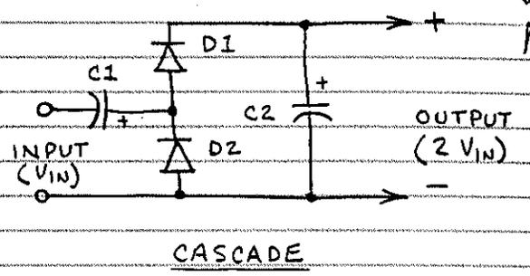
THESE CIRCUITS APPROXIMATELY DOUBLE AN INCOMING AC VOLTAGE. THE OUTPUT IS DC. USE CAPACITORS AND DIODES RATED FOR TWICE THE INPUT VOLTAGE. OUTPUT RIPPLE CAN BE REDUCED BY USING LARGE VALUES FOR C1 AND C2.
