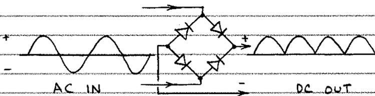
THIS 4-DIODE "NETWORK" (OR BRIDGE RECTIFIER) RECTIFIES BOTH HALVES OF AN AC SIGNAL.
