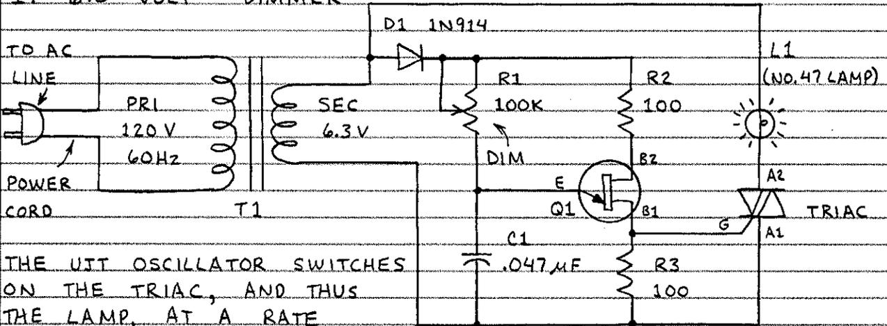
THE UJT OSCILLATOR SWITCHES ON THE TRIAC, AND THUS THE LAMP, AT A RATE CONTROLLED BY R1.
