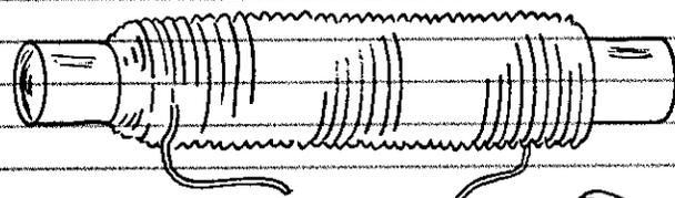
□ ELECTROMAGNET — INSERT A STEEL NAIL IN THE COIL, CONNECT THE LEADS TO A 9-VOLT BATTERY, AND THE NAIL WILL BECOME A MAGNET UNTIL THE POWER IS DISCONNECTED. (IT MAY RETAIN SOME MAGNETISM.)
