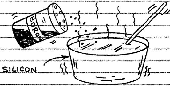
□ P & N SPICED SILICON LOAF — BORON, PHOSPHORUS AND CERTAIN OTHER ATOMS CAN JOIN WITH SILICON ATOMS TO FORM CRYSTALS. HERS'S THE CATCH: A BORON ATOM HAS ONLY THREE ELECTRON IN ITS OUTER SHELL. AND A PHOSPHORUS ATOM HAS FIVE ELECTRONS IN ITS OUTER SHELL. SILICON WITH EXTRA PHOSPHORUS ELECTRONS IS CALLED N-TYPE SILICON (N=NEGATIVE). SILICON WITH ELECTRON DEFICIENT BORON ATOMS IS CALLED P-TYPE SILICON (P= POSITIVE).
