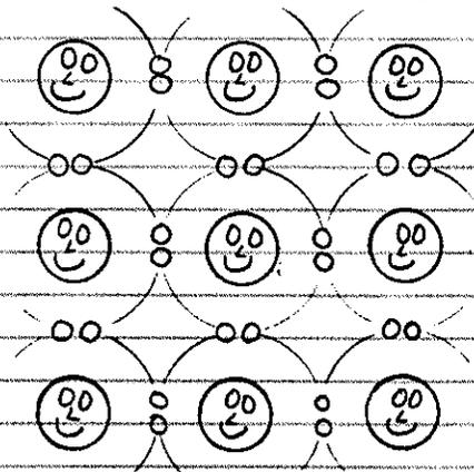
A CLUSTER OF SILICON ATOMS SHARING OUTER ELECTRONS FORMS A REGULAR ARRANGEMENT CALLED A CRYSTAL.
