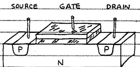
□ MOSFET OPERATION — ALL MOSFETS ARE N-TYPE OR P-TYPE. UNLIKE THE JUNCTION FET, THE GATE OF A MOSFET HAS NO ELECTRICAL CONTACT WITH THE SOURCE AND DRAIN. A GLASS-LIKE LAYER OF SILICON-DIOXIDE (AN INSULATOR) SEPARATES THE GATE'S METAL CONTACT FROM THE REST OF THE TRANSISTOR.
