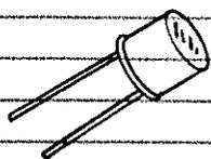
ALL DIODES RESPOND TO SOME DEGREE WHEN ILLUMINATED BY LIGHT. DIODES DESIGNED SPECIFICALLY TO DETECT LIGHT ARE CALLED PHOTODIODES. THEY INCLUDE A GLASS OR PLASTIC WINDOW THROUGH WHICH THE LIGHT ENTERS. OFTEN THEY HAVE A LARGE, EXPOSED JUNCTION REGION. SILICON MAKES GOOD PHOTODIODES.
