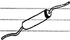
A FOUR-LAYER DIODE IS AN SCR WITHOUT A GATE. IT SWITCHES DC VOLTAGE.
