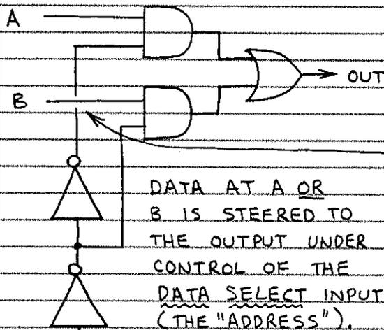
THIS CIRCUIT CAN BE EXPANDED TO SELECT: INCLUDE MANY L SELECTS A MORE INPUTS H SELECTS B AND ADDRESSES.
