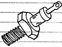
FUNCTIONALLY IDENTICAL TO SMALL SIGNAL DIODES, POWER RECTIFIERS CAN HANDLE MUCH MORE CURRENT. THEY ARE INSTALLED IN LARGE METAL PACKAGES THAT SOAK UP EXCESS HEAT AND TRANSFER IT TO A METAL HEAT SINK. USED MAINLY IN POWER SUPPLIES.
