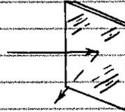
A GLASS MICROSCOPE SLIDE MAKES A GOOD BEAM SPLITTER. (EACH SURFACE REFLECTS 4%.)
