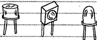
THESE PHOTODIODES HAVE VERY FAST RESPONSE TIMES WHEN USED IN THE REVERSE-BIASED PHOTOCONDUCTIVE MODE.
