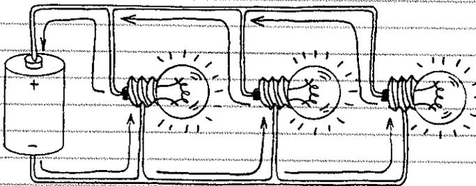
A PARALLEL CIRCUIT IS FORMED WHEN TWO OR MORE COMPONENTS ARE CONNECTED SO CURRENT CAN FLOW THROUGH ONE COMPONENT WITHOUT HAVING FIRST TO FLOW THROUGH ANOTHER.
