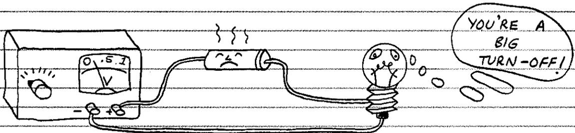
2. IF THE FORWARD CURRENT BECOMES EXCESSIVE, THE SEMICONDUCTOR CHIP MAY CRACK OR MELT! AND THE CONTACTS MAY SEPARATE. IF THE CHIP MELTS, THE DIODE MAY SUDDENLY CONDUCT IN BOTH DIRECTIONS. THE RESULTING HEAT MAY VAPORIZE THE CHIP!
