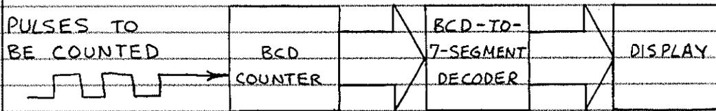
THE BCD COUNTER ADVANCES ONE COUNT FOR EACH INCOMING PULSE. WHEN THE COUNT REACHES 1001 (DECIMAL 9), THE COUNTER RECYCLES TO 0000. THE DECODER ACTIVATES THE APPROPRIATE SEGMENTS OF AN LED DISPLAY.
