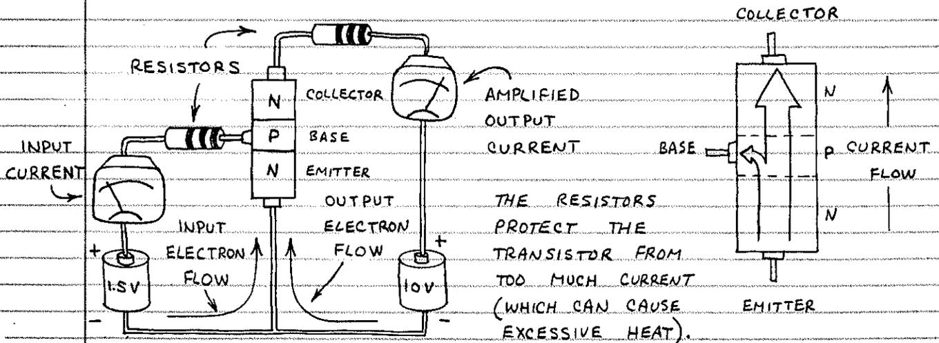
THE RESISTORS PROTECT THE TRANSISTOR FROM TOO MUCH CURRENT (WHICH CAN CAUSE EXCESSIVE HEAT).
