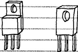
THESE SCRS SWITCH UP TO 10- AMPERES AT UP TO SEVERAL HUNDRED VOLTS. ONE COMMON USE IS SOLID- STATE SWITCHING FOR AUTO ENGINES.
