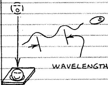
REMEMBER, PHOTONS ACT LIKE WAVES. THE DISTANCE BETWEEN CRESTS IS THE WAVELENGTH. ELECTRONS EXCITED TO HIGHER ENERGY LEVELS EMIT PHOTONS WITH SHORTER WAVELENGTHS THAN ELECTRONS EXCITED TO LOWER LEVELS.
