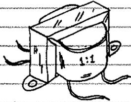
USED TO ISOLATE DIFFERENT PARTS OF A CIRCUIT AND TO PROVIDE PROTECTION FROM ELECTRICAL SHOCK.
