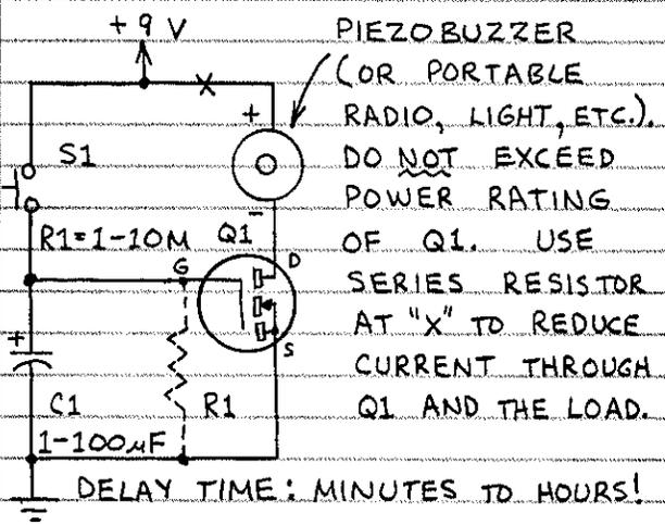
DELAY TIME: MINUTES TO HOURS! CLOSE AND THEN OPEN S1 TO ACTIVATE BUZZER. AFTER C1 DISCHARGES INTERNALLY OR THROUGH R1 (OPTIONAL), Q1 TURNS OFF AND SILENCES THE BUZZER. LONG DELAYS POSSIBLE.
