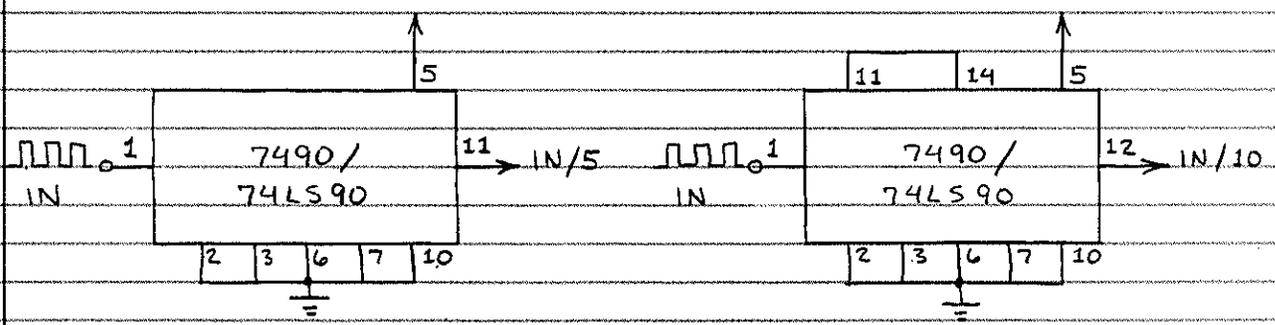
DIVIDES INCOMING "TRAIN" OF PULSES BY 5. OK TO USE AT INPUT OF CIRCUIT ABOVE.
