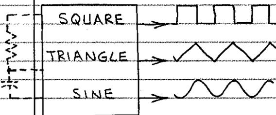
THESE IC'S GENERATE VARIOUS KINDS OF OUTPUT WAVES SUCH AS THOSE SHOWN HERE. THE FREQUENCY OF THE WAVES CAN BE CONTROLLED BY AN EXTERNAL RC CIRCUIT.
