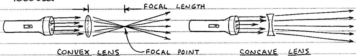
CONVEX LENSES ARE OFTEN USED IN CONJUNCTION WITH SEMI-CONDUCTOR LIGHT SOURCES AND DETECTORS. FOR EXAMPLE, THEY CAN COLLECT AND FOCUS LIGHT ONTO A MINIATURE DETECTOR.
