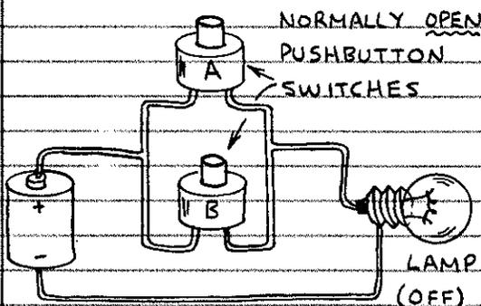
THE LAMP GLOWS ONLY WHEN SWITCH A OR SWITCH B OR BOTH SWITCHES A AND B ARE CLOSED. HERE'S THE TRUTH TABLE:
