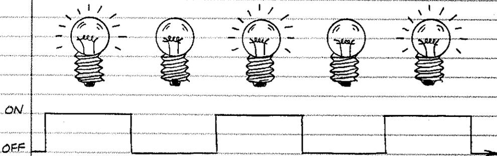
THE FLASHES OF THE LAMP CAN BE REPRESENTED BY A DIAGRAM LIKE THIS...
