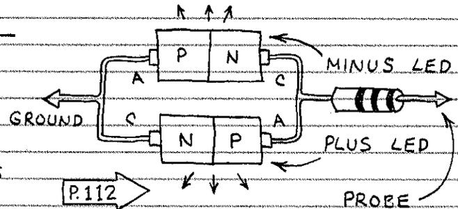
□ PULSED LED — WHEN OPERATED CONTINUOUSLY, AN INFRARED LED MIGHT HAVE A MAXIMUM CURRENT OF 100-MILLIAMPERES. WHEN DRIVEN BY BRIEF PULSES OF CURRENT, THE SAME LED MAY SAFELY ACCEPT HUGE 10-AMPERE PULSES!
