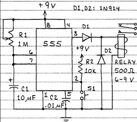
PRESS S1 MOMENTARILY TO START TIMING CYCLE. RELAY WILL BE ACTUATED (PULLED IN) UNTIL CYCLE IS COMPLETE. R1 AND C1 CONTROL LENGTH OF TIME DELAY. USE VERY LARGE VALUE FOR C1 TO GET LONG DELAYS. CIRCUIT WILL RESPOND TO LOGIC PULSES, TOO.
