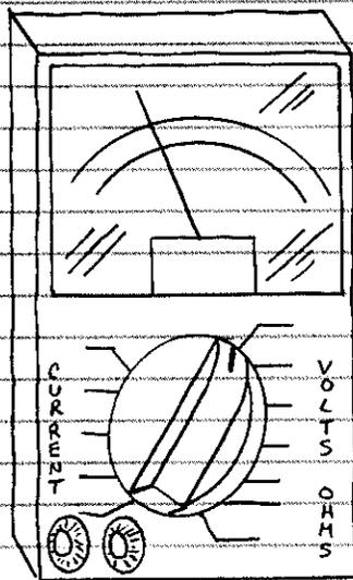
YOU CAN EASILY MEASURE AC AND DC VOLTAGE AND CURRENT WITH AN INSTRUMENT CALLED THE MULTIMETER. ANALOG MULTIMETERS USE A MOVING COIL METER. DIGITAL MULTIMETERS HAVE A DIGITAL READOUT. THE MULTIMETER IS THE SINGLE MOST IMPORTANT ELECTRONIC TEST INSTRUMENT.
