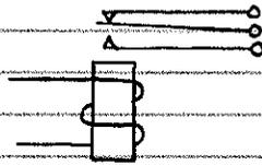
THIS IS THE SYMBOL FOR A RELAY WITH SPDT CONTACTS.
