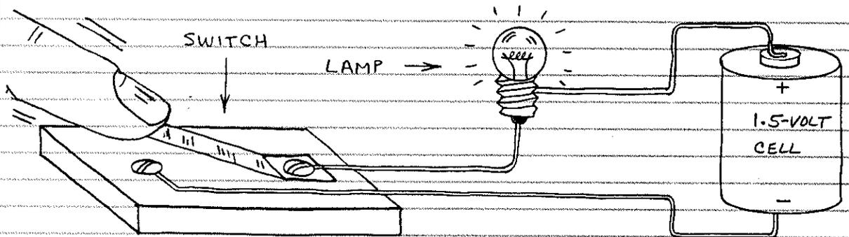
THIS SIMPLE CIRCUIT IS REALLY MORE USEFUL THAN IT FIRST APPEARS BECAUSE IT CAN SEND INFORMATION BY CONVERTING A PLANNED SEQUENCE OF SWITCH CLOSURES INTO FLASHES OF LIGHT.
