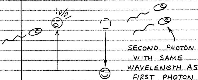
EXCITED ELECTRONS CAN RESUME THEIR NORMAL LEVEL SPONTANEOUSLY. OR A PHOTON WITH THE PROPER WAVELENGTH CAN STIMULATE AN EXCITED ELECTRON TO RETURN TO ITS NORMAL LEVEL.
