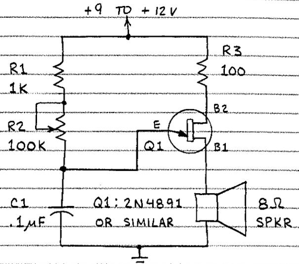
THIS CIRCUIT IS IDENTICAL IN PRINCIPLE TO THE ADJACENT CIRCUIT. C1 IS MUCH SMALLER TO SPEED UP THE CHARGE-DISCHARGE CYCLE. THE RESULT IS AN AUDIO FREQUENCY TONE WHICH IS EMITTED BY THE SPEAKER. THIS CIRCUIT CAN BE EXPANDED (SEE BELOW).
