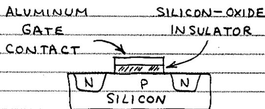
A POSITIVE GATE VOLTAGE ATTRACTS ELECTRONS TO THE REGION BELOW THE GATE. THIS CREATES A THIN N-TYPE CHANNEL IN THE P-TYPE SILICON BETWEEN THE SOURCE AND DRAIN. CURRENT CAN THEN FLOW THROUGH THE CHANNEL. THE GATE VOLTAGE DETERMINES THE RESISTANCE OF THE CHANNEL.
