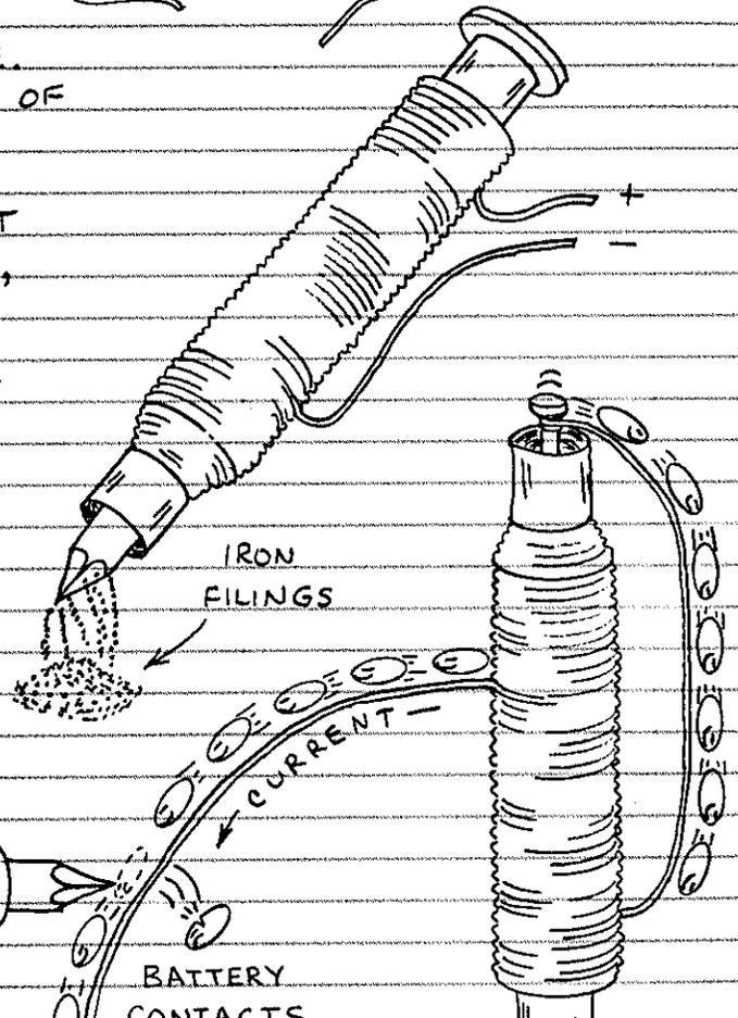
□ MOTOR — MAYBE NOT YOUR IDEA OF A MOTOR, BUT THIS ELEGANT APPARATUS QUALIFIES UNDER THE DICTIONARY DEFINITION. USE A LIGHT WEIGHT NAIL. SECURE ONE COIL LEAD TO NAIL. ADJUST HEIGHT OF COIL UNTIL NAIL JUMPS UP AND DOWN.
