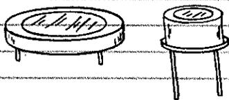
THOUGH SLOWER RESPONDING THAN SMALL AREA PHOTODIODES, THEIR LARGE AREA PROVIDES HIGH SENSITIVITY.
