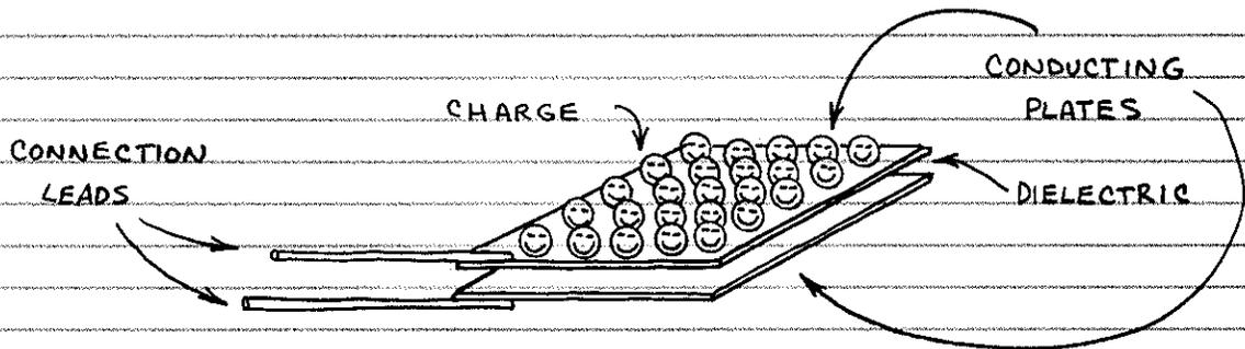
THE DIELECTRIC CAN BE PAPER, PLASTIC FILM, MICA, GLASS, CERAMIC, AIR OR A VACUUM. THE PLATES CAN BE ALUMINUM DISCS, ALUMINUM FOIL OR A THIN FILM OF METAL APPLIED TO OPPOSITE SIDES OF A SOLID DIELECTRIC. THE CONDUCTOR-DIELECTRIC-CONDUCTOR SANDWICH CAN BE ROLLED INTO A CYLINDER OR LEFT FLAT. MORE ABOUT TYPES OF CAPACITORS LATER.
