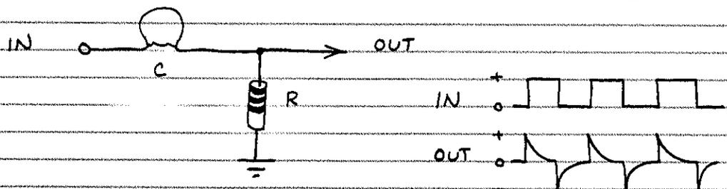
THIS CIRCUIT PRODUCES SYMMETRICAL OUTPUT WAVES WITH SHARP POSITIVE AND NEGATIVE PEAKS. IT'S USED TO MAKE NARROW PULSE GENERATORS FOR TELEVISION RECEIVERS AND TO TRIGGER DIGITAL LOGIC CIRCUITS.
