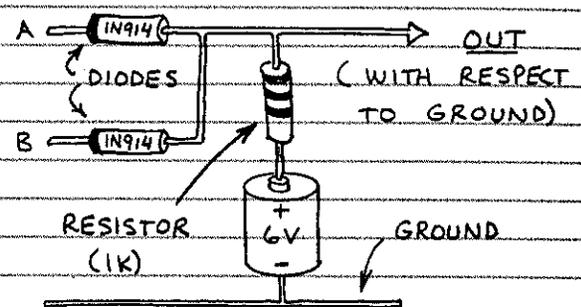
WHEN THE INPUT VOLTAGE AT A OR B IS MORE POSITIVE THAN GROUND, IT PASSES THROUGH THE FORWARD BIASED DIODE(S) AND APPEARS AT THE OUTPUT. OTHERWISE THE OUTPUT IS AT OR NEAR GROUND. THE TRUTH TABLE IS VALID FOR INPUTS OF 0 VOLT (0 OR LOW) AND +6 VOLTS (1 OR HIGH).
