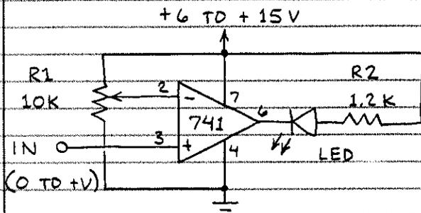
WHEN THE INPUT VOLTAGE IS 0, THE LED GLOWS. THE LED SWITCHES OFF WHEN THE INPUT VOLTAGE RISES TO A LEVEL DETERMINED BY R1. EXCHANGE CONNECTIONS TO PINS 2 AND 3 TO REVERSE OPERATING MODE.
