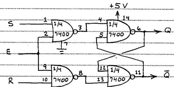
FUNCTIONS AS "RS" FLIP-FLOP WHEN ENABLE (E) IS HIGH.
