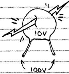
MAKE SURE THE CAPACITOR YOU PLAN TO USE MEETS OR EXCEEDS THE REQUIRED VOLTAGE RATING. OTHERWISE ITS DIELECTRIC MAY BE ZAPPED BY THE STORED CHARGE. THE VOLTAGE RATING IS USUALLY PRINTED ON THE CAPACITOR. V MEANS VOLTS. WV IS WORKING VOLTS (SAME THING).
