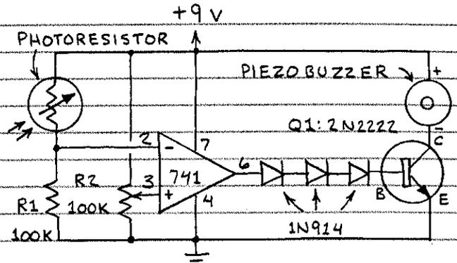
BUZZER SOUNDS WHEN LIGHT FALLS TO LEVEL DETERMINED BY R2. REVERSE CONNECTIONS TO PINS 2 AND 3 TO SOUND TONE WHEN LIGHT INCREASES.
