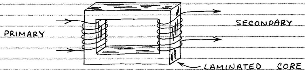
IF THE CURRENT FLOWING THROUGH THE PRIMARY COIL IS FLUCTUATING, THEN A CURRENT WILL BE INDUCED INTO THE SECONDARY WINDING. A STEADY (DC) CURRENT WILL NOT BE TRANSFERRED FROM ONE COIL TO THE OTHER.
