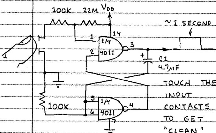
C1 CONTROLS LENGTH OF OUTPUT PULSE.
