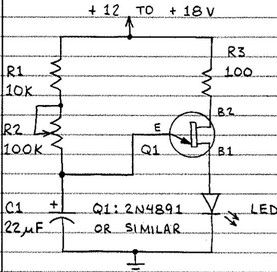
EACH TIME THE UJT (Q1) TURNS ON, THE CHARGE ON C1 IS "DUMPED" THROUGH THE LED. THE LED FLASHES IN RESPONSE. BETWEEN FLASHES, THE LED GLOWS DIMLY. R2 CONTROLS FLASH RATE AND CAN BE SET FOR ONE FLASH PER SECOND (TIME BASE ROLE).
