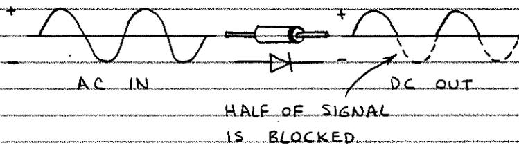
AN UNDULATING (AC) SIGNAL (OR VOLTAGE) IS RECTIFIED INTO A SINGLE POLARITY (DC) SIGNAL (OR VOLTAGE).
