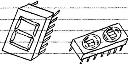
MANY KINDS OF LED READOUTS CAPABLE OF DISPLAYING DIGITS AND CHARACTERS ARE AVAILABLE. THEY ARE MORE RUGGED THAN LIQUID CRYSTAL DISPLAYS, BUT THEY USE MUCH MORE CURRENT.
