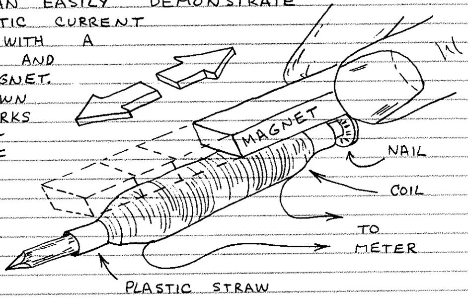
THROUGH THE COIL AND STROKE THE MAGNET BACK AND FORTH ACROSS THE COIL. THE METER WILL INDICATE A FEW MICROAMPERES EACH STROKE. THE POLARITY (DIRECTION) OF THE CURRENT WILL REVERSE ON THE BACK STROKES. WANT A READY-MADE GENERATOR? JUST ROTATE THE SHAFT OF A SMALL DC MOTOR.
