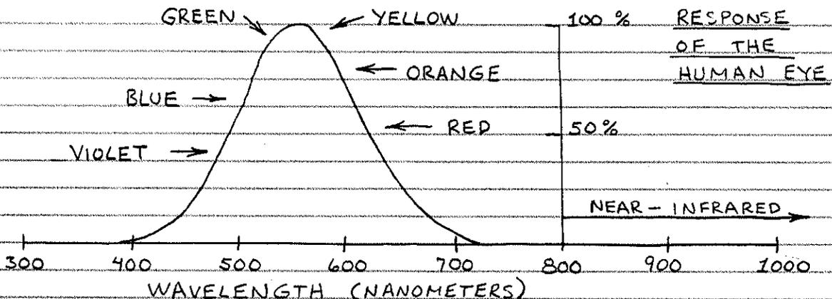
MANY PHOTONIC SEMICONDUCTORS EMIT OR DETECT NEAR-INFRARED RADIATION. SILICON, FOR EXAMPLE, CAN DETECT VISIBLE LIGHT. BUT IT IS MOST SENSITIVE TO NEAR-INFRARED AT ABOUT 880 nm. BECAUSE SO MANY PHOTONIC COMPONENTS CAN OPERATE IN BOTH THE VISIBLE AND NEAR-INFRARED, IT'S COMMON TO REFER TO NEAR-INFRARED AS LIGHT.
