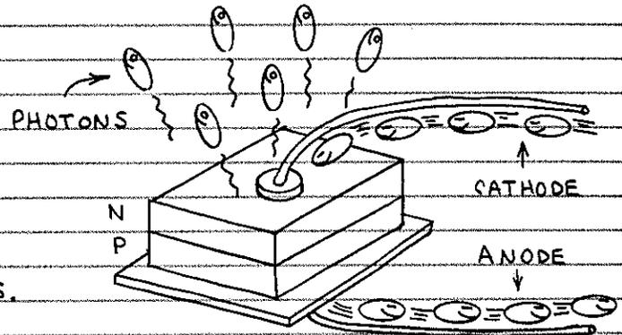
□ LED OPERATION— THE FORWARD VOLTAGE ACROSS A DIODE MUST EXCEED A THRESHOLD LEVEL BEFORE A CURRENT CAN CROSS THE JUNCTION. FOR SILICON, WHICH EMITS A TINY AMOUNT OF NEAR-INFRARED, THE THRESHOLD IS 0.6-VOLT. FOR GALLIUM ARSENIDE, WHICH EMITS CONSIDERABLE NEAR-INFRARED, THE THRESHOLD IS 1.3-VOLTS. THIS VOLTAGE EXCITES THE ELECTRONS. WHEN THE ELECTRONS CROSS THE JUNCTION AND COMBINE WITH HOLES, THEY EMIT PHOTONS.
