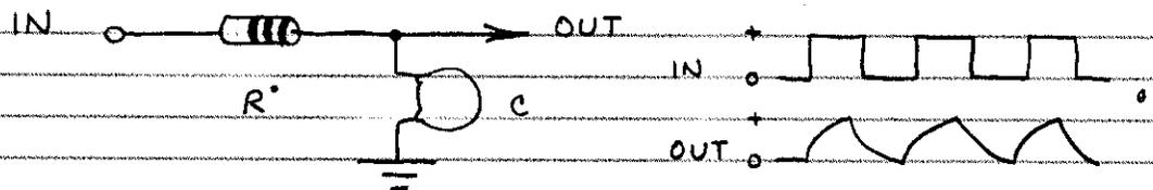
IF THE INPUT PULSES ARE SPEEDED UP, THE OUTPUT WAVEFORMS (OFTEN CALLED A SAWTOOTH) WILL NOT REACH THEIR FULL HEIGHT (AMPLITUDE). IT'S EASY TO DESIGN AN AMPLIFIER THAT IGNORES WAVES WITH LESS THAN A DESIRED AMPLITUDE. THEREFORE, THE INTEGRATOR CAN FUNCTION AS A FILTER WHICH PASSES ONLY SIGNALS BELOW A CERTAIN FREQUENCY.
