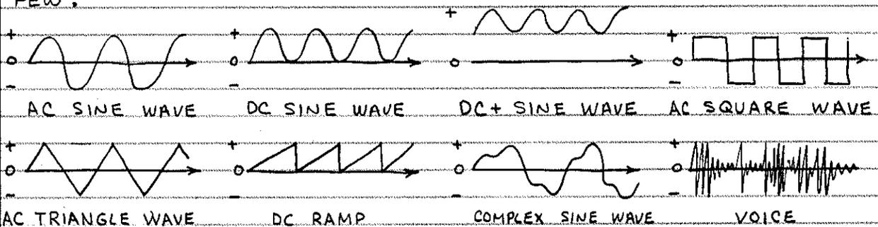
□ SIGNALS — A SIGNAL IS A PERIODIC WAVEFORM THAT CONVEYS INFORMATION. THE PROCESS THAT GENERATES THE WAVEFORM IS CALLED MODULATION. SIGNALS CAN BE AC, DC OR AC RIDING ON A DC LEVEL. THEIR ENEMY IS...
