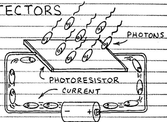
☐ PHOTORESISTOR OPERATION. THIS PANEL SHOWS HOW A PHOTON CREATES A HOLE-ELECTRON PAIR. AN EXTERNAL VOLTAGE WILL FORCE THE HOLE AND ELECTRON TO MOVE.
