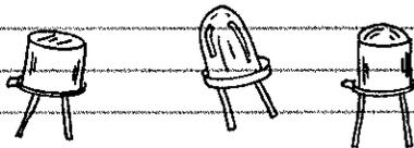
INFRARED LEDs SHOULD BE CALLED INFRARED EMITTING DIODES. THEY ARE USED TO TRANSMIT INFORMATION. THEY ARE ALSO USED IN INTRUSION ALARMS, REMOTE CONTROL DEVICES, ETC. A SPECIAL KIND OF INFRARED LED IS THE DIODE LASER. SOME EMIT SEVERAL WATTS!
