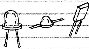
THESE INEXPENSIVE LEDs ARE USED AS INDICATOR LIGHTS. CERTAIN RED LEDs ARE USED TO TRANSMIT INFORMATION. MOST ARE ENCAPSULATED IN EPOXY.
