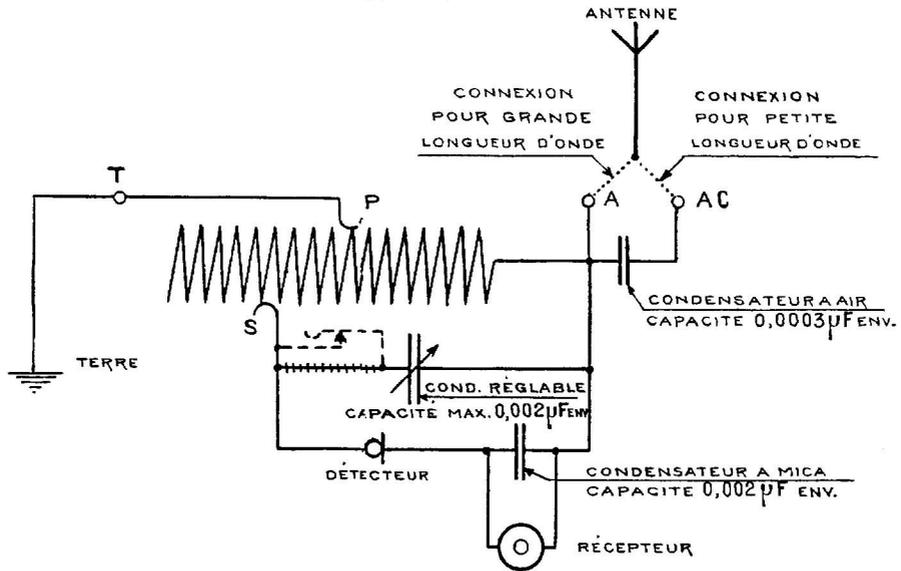
+++++ SCHÉMA AVEC CONDENSATEUR SANS COUPURE
