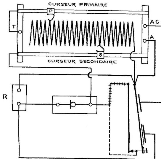
+++++ CÂBLAGE AVEC CONDENSATEUR SANS COUPURE
