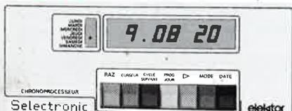
**HORLOGE PROGRAMMABLE AUTOMATIQUE PAR RÉCEPTION DE SIGNAUX CODÉS "FRANCE-INTER" RÉCEPTEUR SANS MISE AU POINT**
