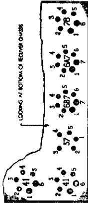
Fig. 12. Location of Socket Terminals for Measuring Voltages.
