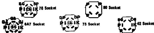
Terminal Arrangement of Tube Sockets Viewed From Under Side of Chassis
