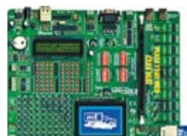
Thanks to many features **UNI-DS3** is the world's easiest to use development board for different types of microcontrollers. The system supports **PIC**, **dsPIC**, **AVR**, **8051**, **ARM** and **PSOC** microcontrollers with a large number of peripherals. In order to continue working with different chip in the same development environment, you just need to switch a card. You can choose between **USB** or **External Power supply**. Each MCU card has its own **USB 2.0** programmer!
