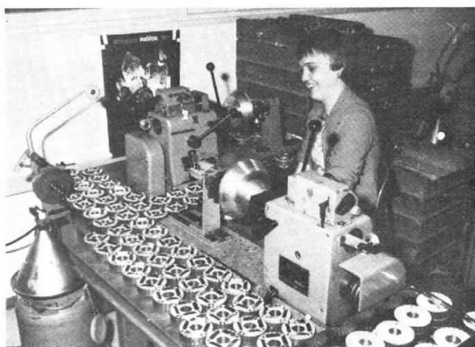
Photo 8. - Bobinage des stators.
