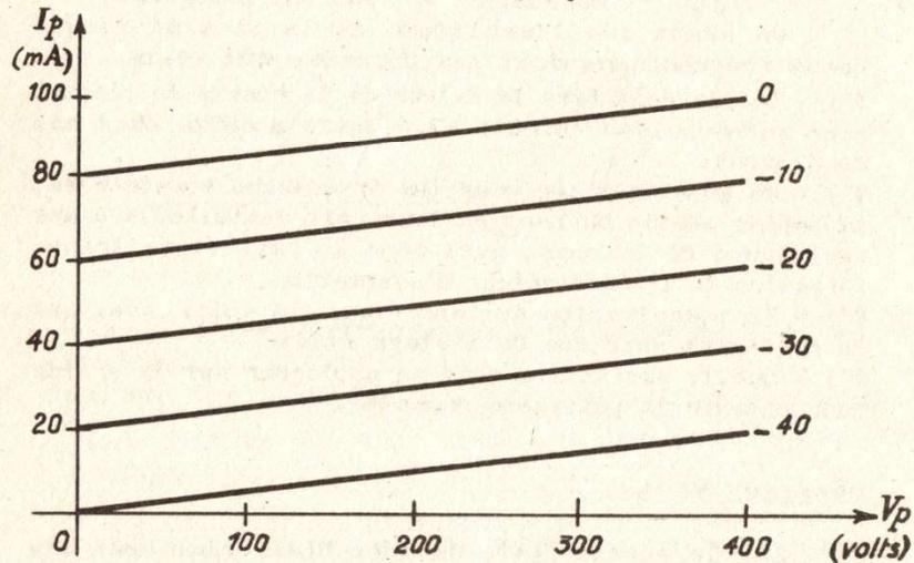
La charge optimum de plaque à plaque  $2Z_0 = 8000$  ohms
