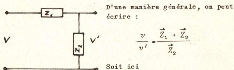
$$\frac{v}{v'} = \frac{\sqrt{(R + R')^2 + \left(L\omega - \frac{1}{C\omega}\right)^2}}{\frac{1}{C\omega}}$$
