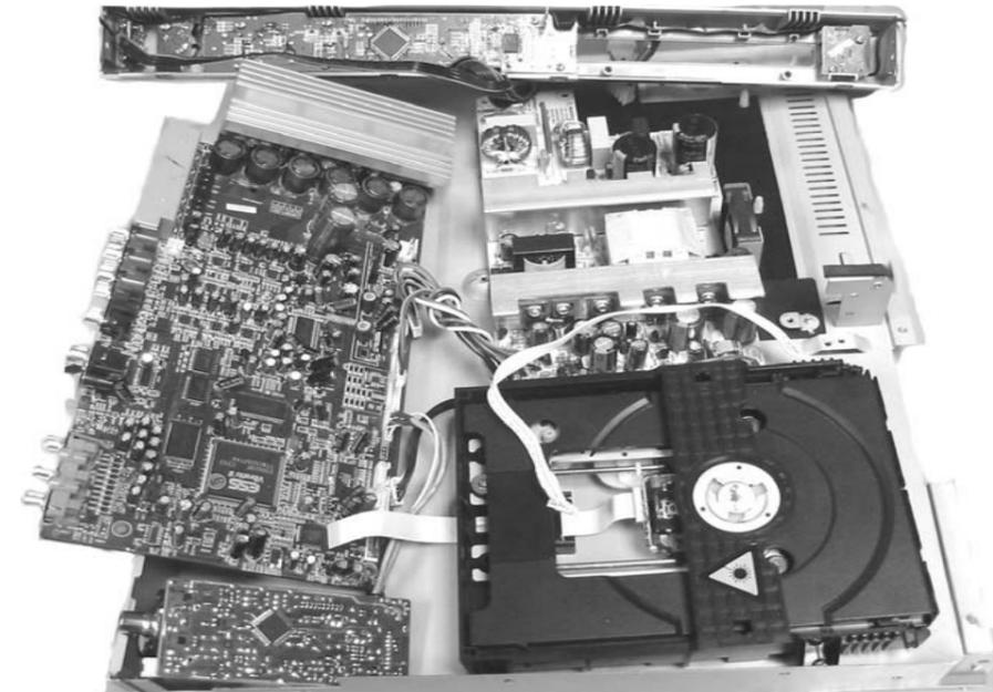
Note: In some service positions the components or copper patterns of one board may risk touching its neighbouring pc boards or metallic parts. To prevent such short-circuit use a piece of hard paper or other insulating material between them.
