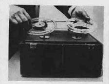
Lift both reels carefully, trying not to snag the tape on control levers and knobs. Keep slight tension on tape to prevent it from unraveiling.
