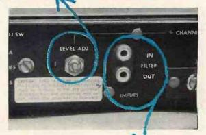
DYNACO STEREO 70 has power takeoff for preamplifier (as does Pilot). Bias is set with a voltmeter and seldom needs readjustment.
