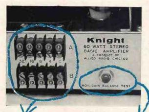
KNIGHT-KIT offers 32-ohm tap so two amplifiers may be strapped in parallel for mono operation.
