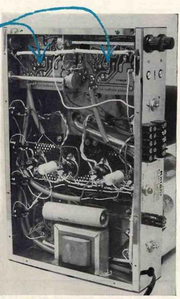
FISHER SA-300 is one of the two amplifiers in this group with input level controls. High sensitivity power amplifiers require such controls to permit great flexibility in preamplifier selection.
