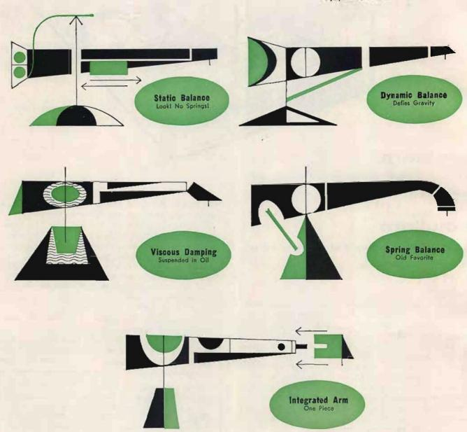
THE most self-effacing of all high fidelity components is the tone arm. Its task is utter passivity. Traveling slowly across the disc, it is propelled not by forces of its own, but limply follows the guiding impetus of the record spiral. It generates no sound of its own. It is, in effect, a "silent partner" in the musical enterprise.
