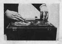
Pick up both reels from their new table top position and thread through the transport. You're now ready to go with the tracks in the opposite sequence: A and C, or B and D.
