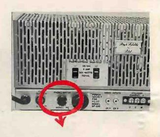
PILOT SA-260 is an amplifier of honest specifications without bravado or undue optimism. The entire electronic circuit is straightforward and although harmonic and IM distortion levels were slightly above the other amplifiers in this test the \$4.260 rates high in stability. Circle above shows connection permitting umplifter to be shut off by automatic switch in many record changers.
