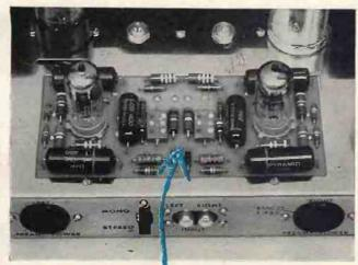
DYNACO STEREO 70 is supplied as a partially assembled kit. All resistors and capacitors are soldered to the circuit board by the manufacturer. Wiring time to complete the amplifier is about five hours. This one printed circuit board holds both voltage amplifiers and phase inverters.
