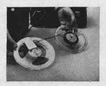
4 Keeping tension on the tape, swing both reels around in an arc so that the positions are reversed.
