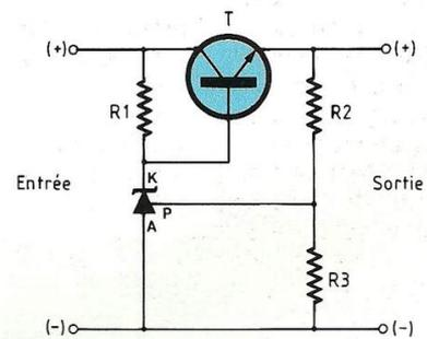
Fig. 14 U<sub>sortie</sub> = 2,5 · [1 + R<sub>2</sub>/R<sub>3</sub>] volts
