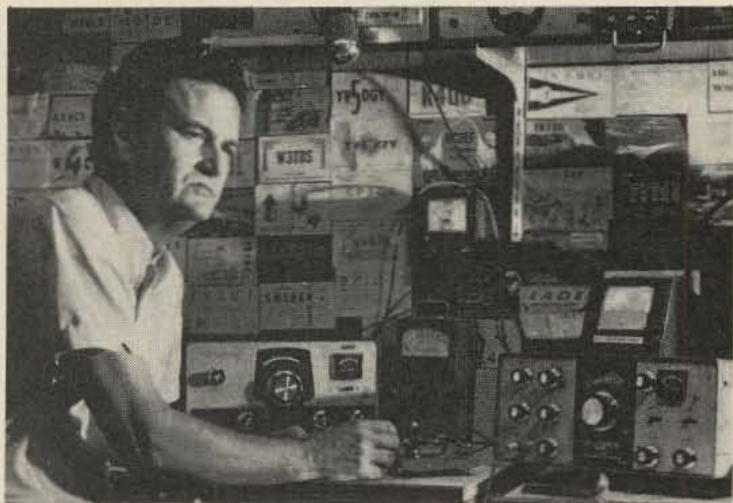
WB4SNC, Albert Coya, at his shack. The equipment is a HW-101 Heathkit, a HW 32 monobander for 20 meters, and a homebrew linear. Other gear shown: homebrew phone patch, frequency counter, keyer, SW R meter, monitor scope, and power supply for both rigs.
