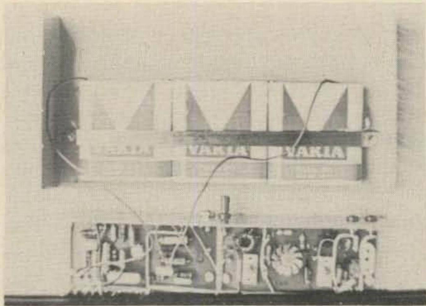
The power supply for the author's portable transceiver consists of three 4.5V flat batteries held in the top cover of the transceiver enclosure.
