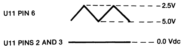
Figure 6-33. AM Level Shifter Waveforms
