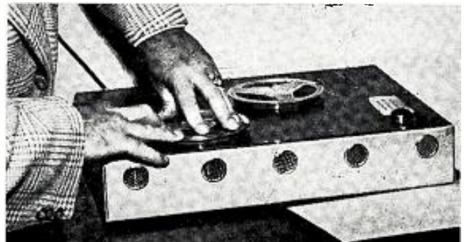
The tank-type Degausser is used in many places where there is a good quantity of erasing to be done, such as recording studios, radio stations, tape libraries, etc. The reels are placed on the panel, rotated and then very slowly withdrawn to complete the erase.
