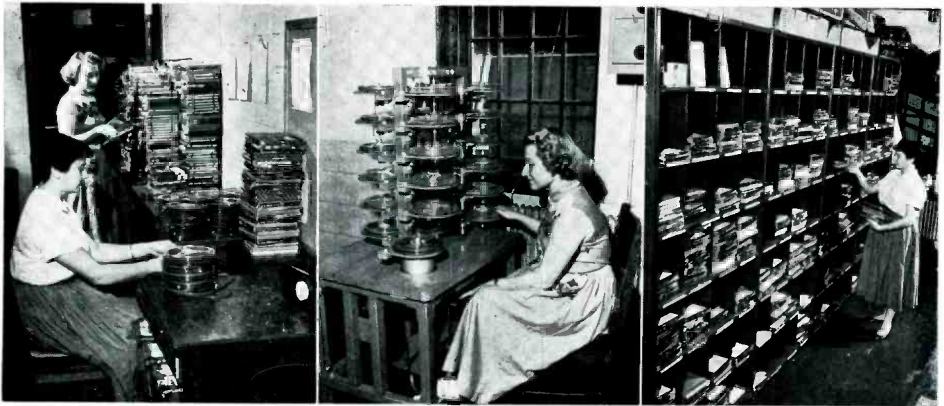
Left to right: Diane Aronovsky, seated, wipes the incoming tapes clean on a Cinema tank-tape eraser, while Kitty Schneider prepares the tapes for re-recording and another trip out. Center, Kitty Schneider makes copies of the programs on the erased tapes. On this mass duplicator, eleven copies of half-hour programs can be made in ten minutes. Right: tapes are sorted by stations.
