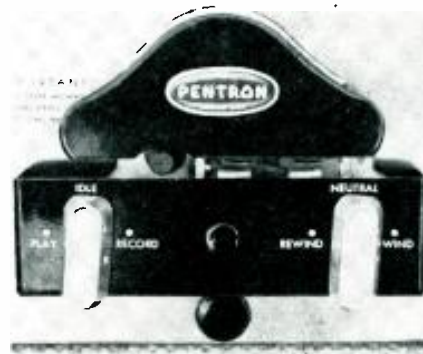
The tape mechanism controls are the familiar 9T3C units which appear on a number of recorders manufactured by Pentron.
