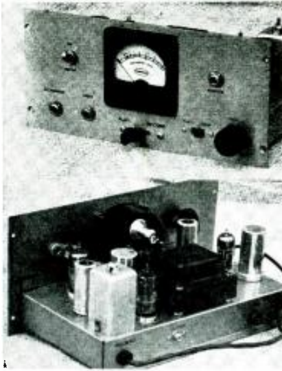
Front and rear views of the HFP-1 preamplifier. The unit is well and simply made and has an illuminated VU meter for recording level.
